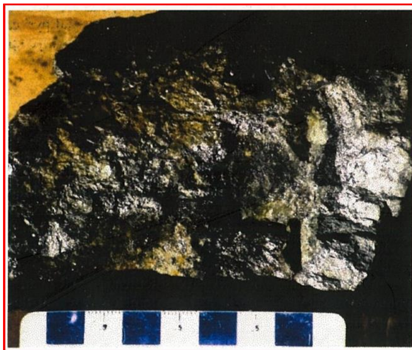
Photo 12. Semi-massive arsenopyrite with quartz – Sandvik showing (8.5 g/t Au – sample 174602). Source: Osmani et al. (2004).
