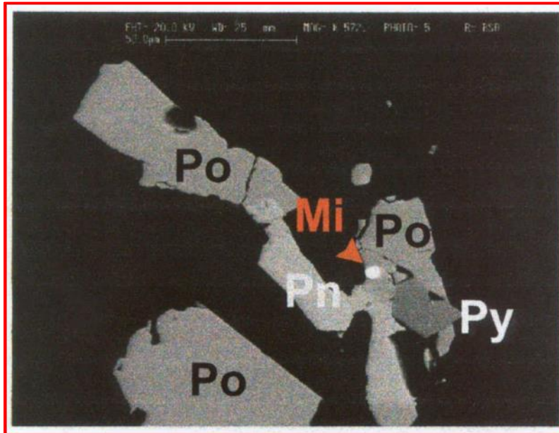
Figure 37. Electron backscatter image of michenerite (Mi) associated with an interstitial sulphide aggregate of pyrrhotite (Po), pentlandite (Pn), and pyrite (Py). The black background is silicate—sample 166092.
