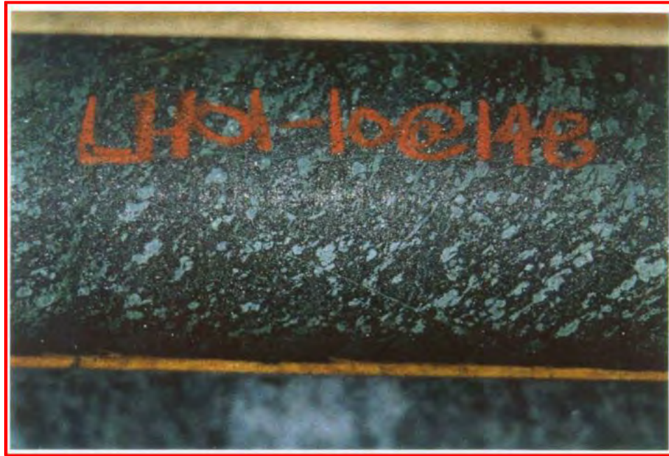
Photo 11. Massive titanomagnetite lens at 148.0 m - drill hole LH01-10, Gabbro Lake.
