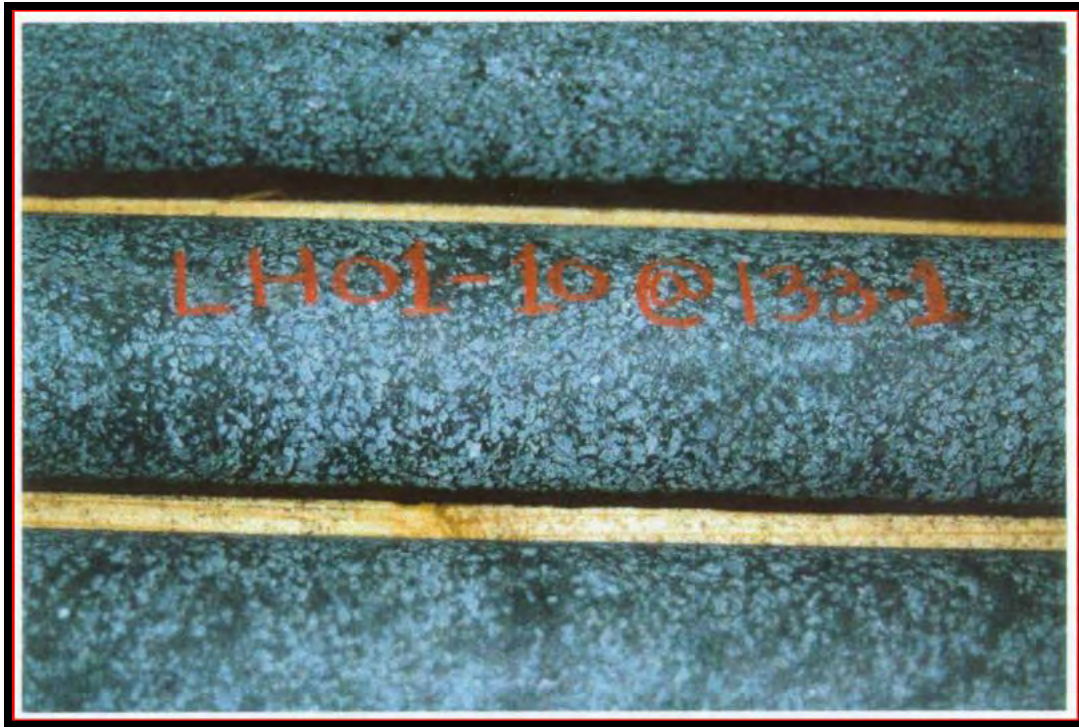
Photo 3. Anorthosite to leucogabbro comprising cumulus plagioclase with intercumulus titanomagnetite and subordinate amphiboles; drill hole LH01-10, Gabbro Lake (Osmani and Samson, 2002).
