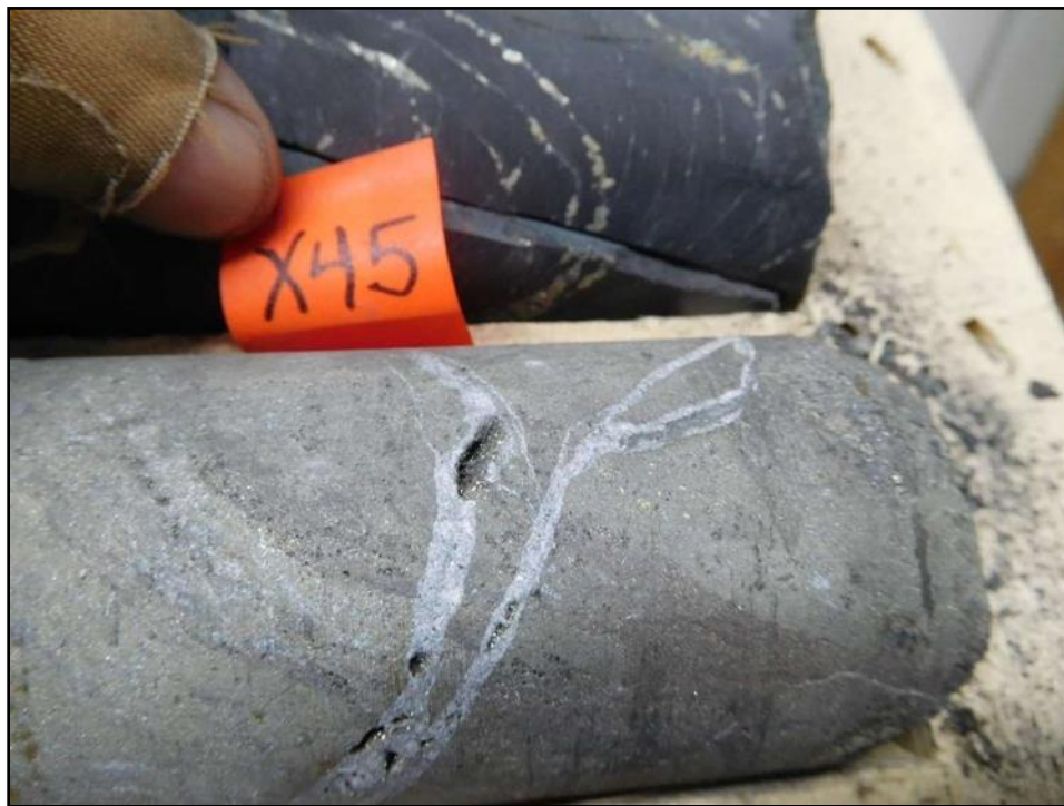
Figure 9. 4 Core pictures for Zn-Cu intersects near 191 m in hole CHA-17-10 (Source Charbonneau, R and Robillard, I, 2017)
