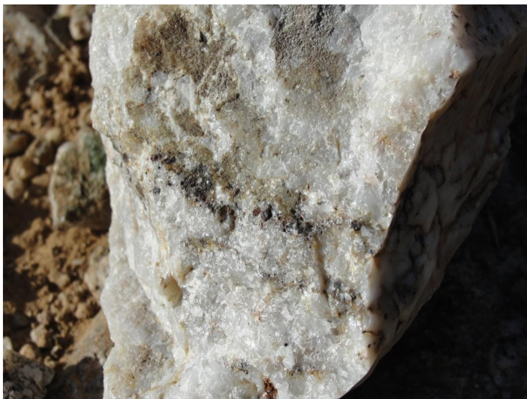
Figure 12-6: Sample Location UT-26. Quartz vein with pyrite layers and possible weathered galena.
