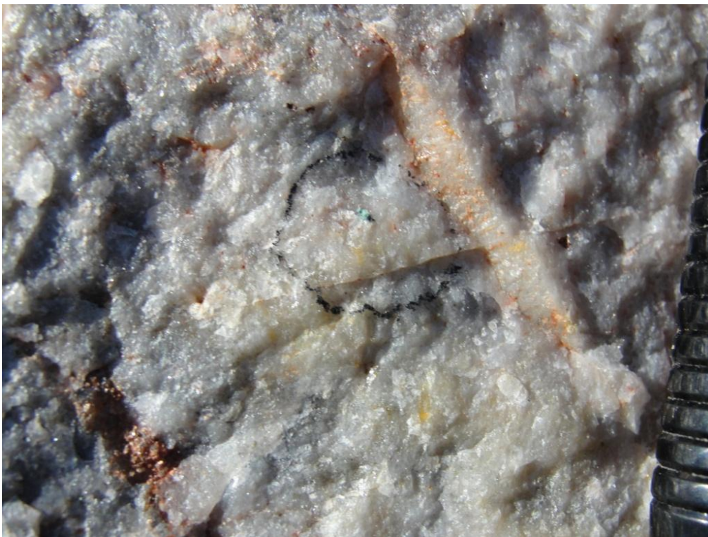
Figure 12-9: Sample location UT-15. Malachite mineralisation in quartzite
