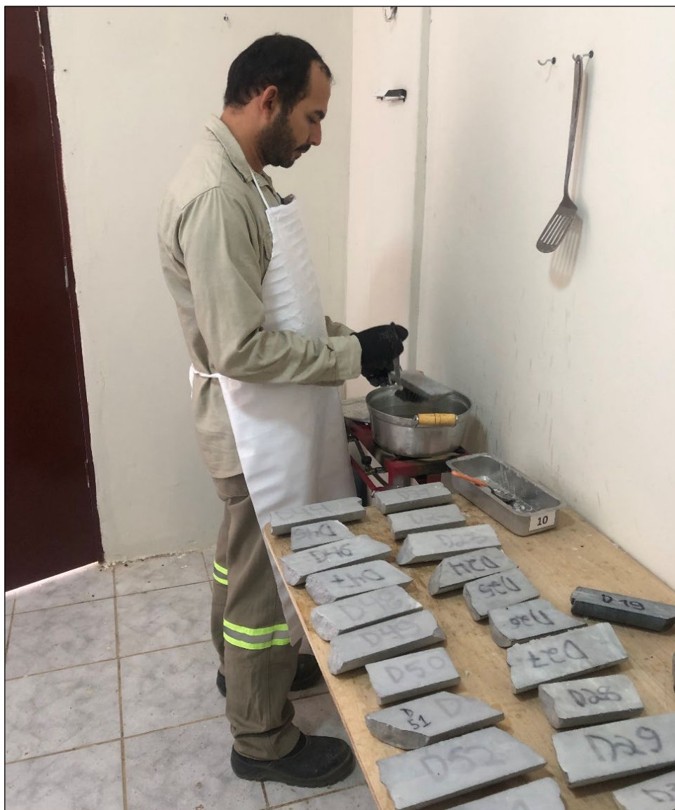
Figure 11-11. Sub-Samples Coated with Wax and Identified with Numbers and Labeled Container for Transportation
