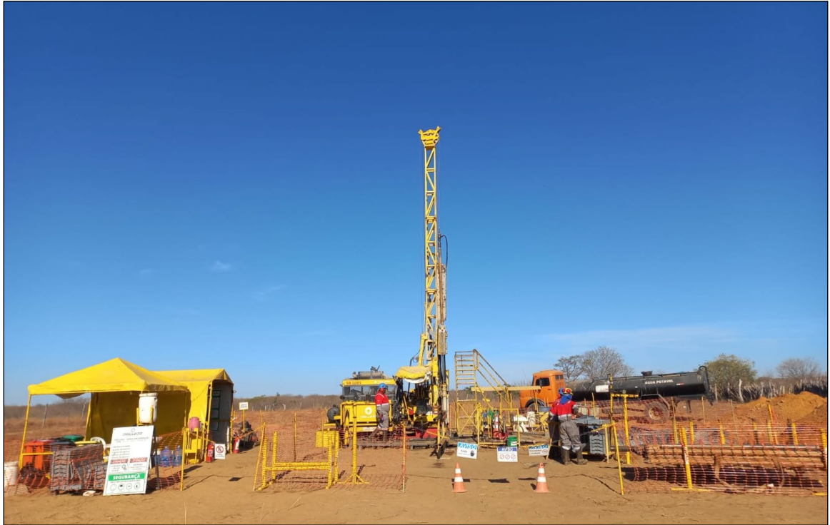
Figure 10-1: Diamond Drilling Rig at Mangueiros Site
