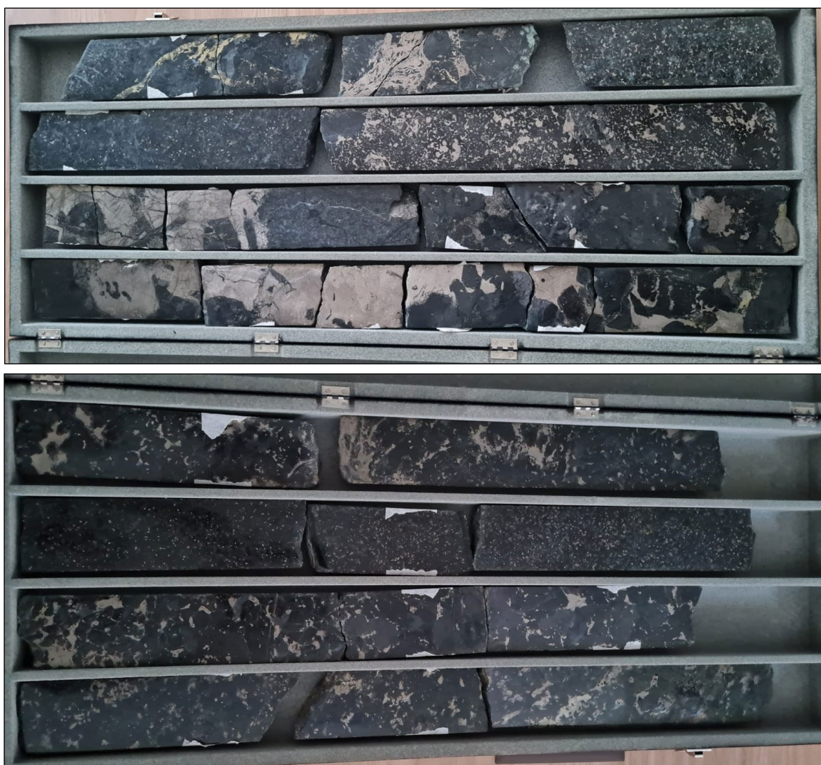
Figure 7-12: Examples of Sulfide Textures from Mangueiros Main and Lagoa da Onça Targets
