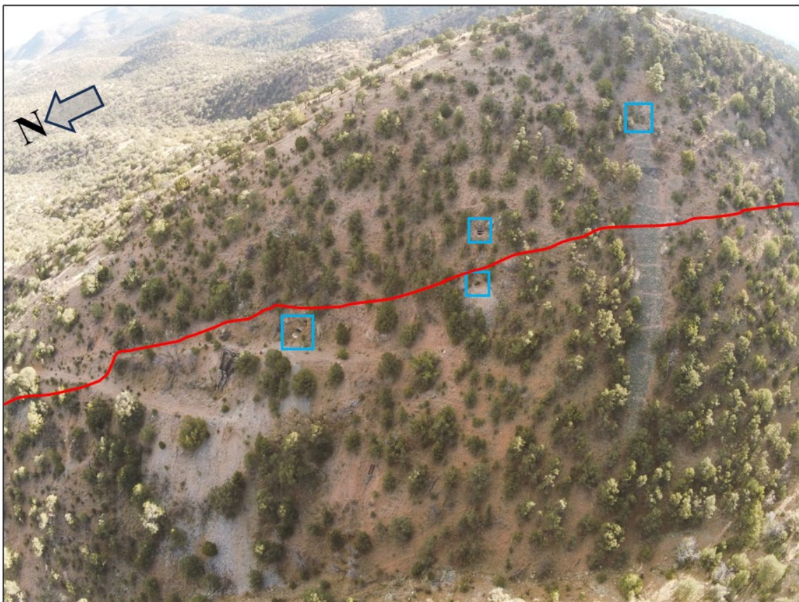
Figure 6-4 - Drone photo of Ivanhoe Mine, surface vein trace indicated by red line and blue squares show adits.
