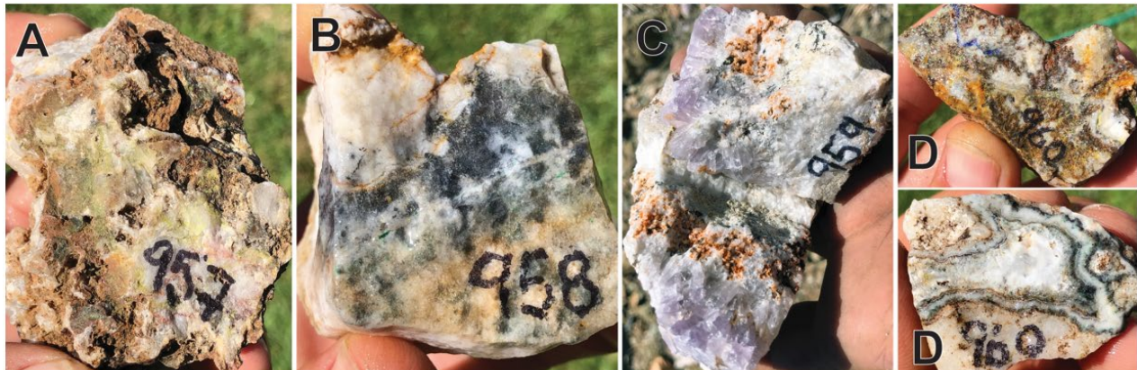
Ore from Ivanhoe-Emporia Mine: A) banded comb qtz w sulphides and open space qtz growth, boiling textures evident, some amethyst, CuOxides, and dark grey qtz zones, with bright green Ag-chlorides; B) sugary white qtz w patches-lines of black sulphides; C) Amethyst Qtz Vein, boiling textures, patches of orange-black oxides, some Bx; D) middle up hill on Emporia Vein; ginguro banding and high-sulphide layers in with minor amethyst.
