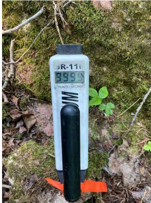
Figure 27: Exploranium GR-110 unit displaying 9999 cps, its maximum reading limit, on a pegmatite outcrop located in a blasted trench on the Bee Lake occurrence UTM co-ordinates 15U 0439293mE, 5521912mN, in the vicinity of a previous old sample SB09. This reading was recorded in 2020 from an earlier site visit by R. Komarechka.
