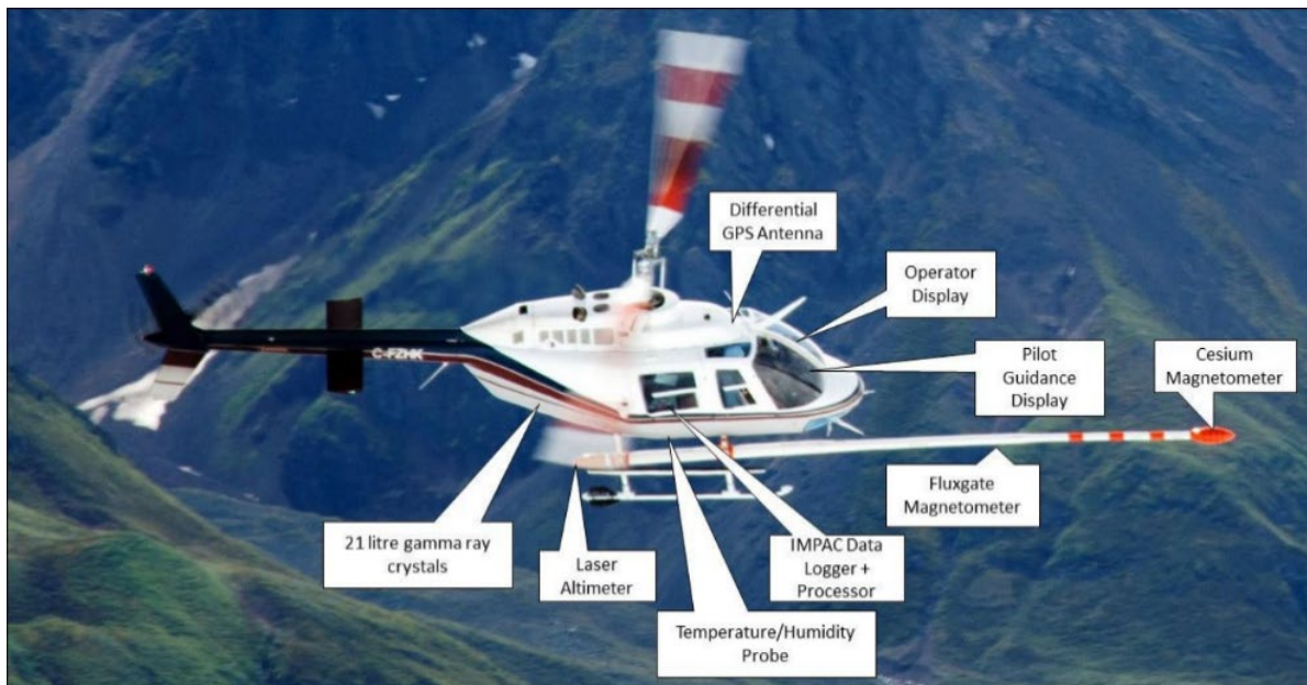
Figure 9-2: Survey helicopter equipped with a magnetic sensor and gamma ray spectrometer
