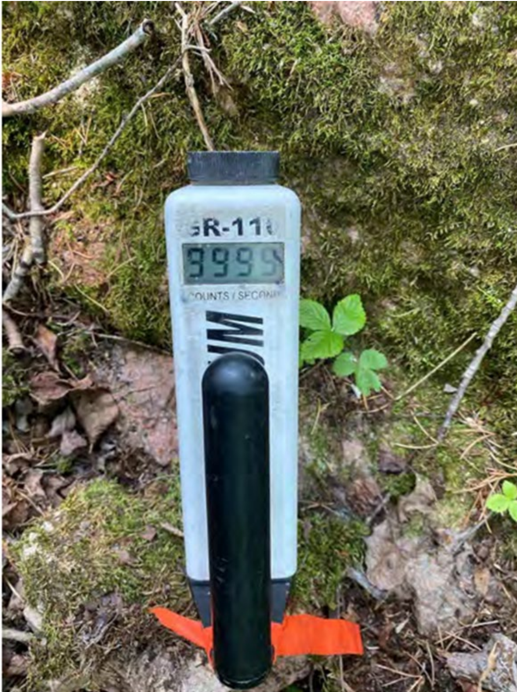
Figure 12-14: Exploranium GR-110 unit displaying 9999 counts per second (cps), its maximum reading limit, on a pegmatite outcrop located in a blasted trench on the Bee Lake Occurrence UTM co-ordinates 15U 0439293mE, 5521912mN, in the vicinity of a previous old sample SB09. This reading was recorded in 2020 from an earlier site visit by R. Komarechka, a QP of this report.
