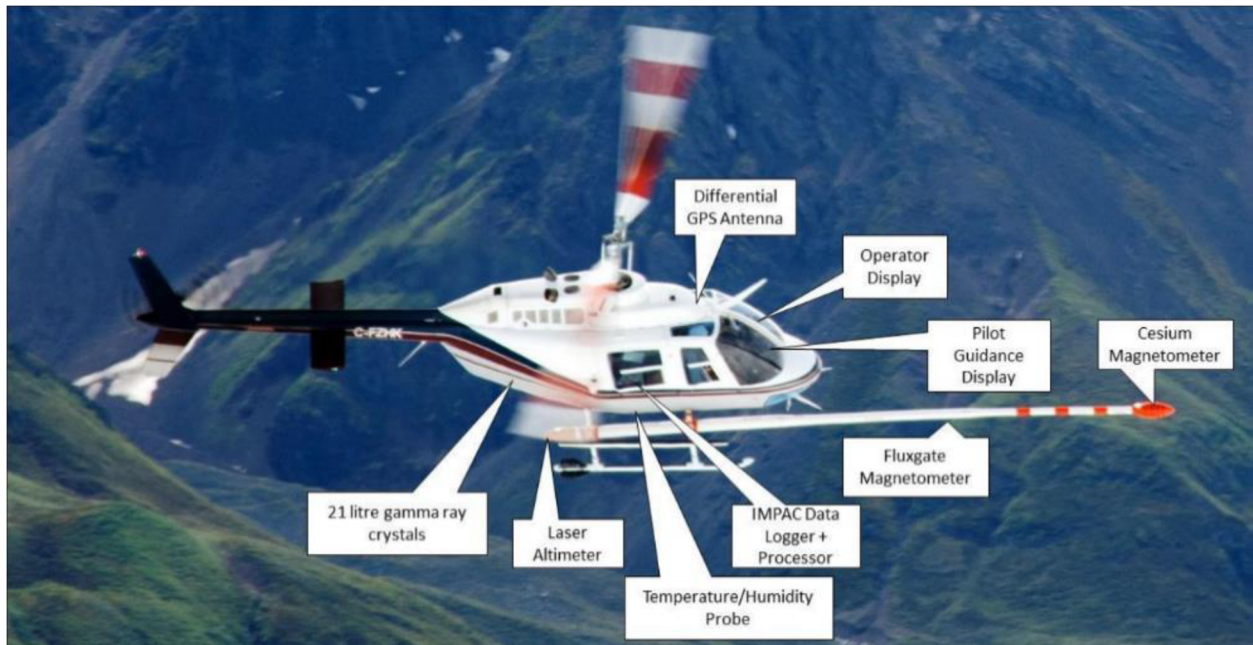
Figure 10: Survey Helicopter Equipped with a Magnetic Sensor and Gamma Ray Spectrometer
