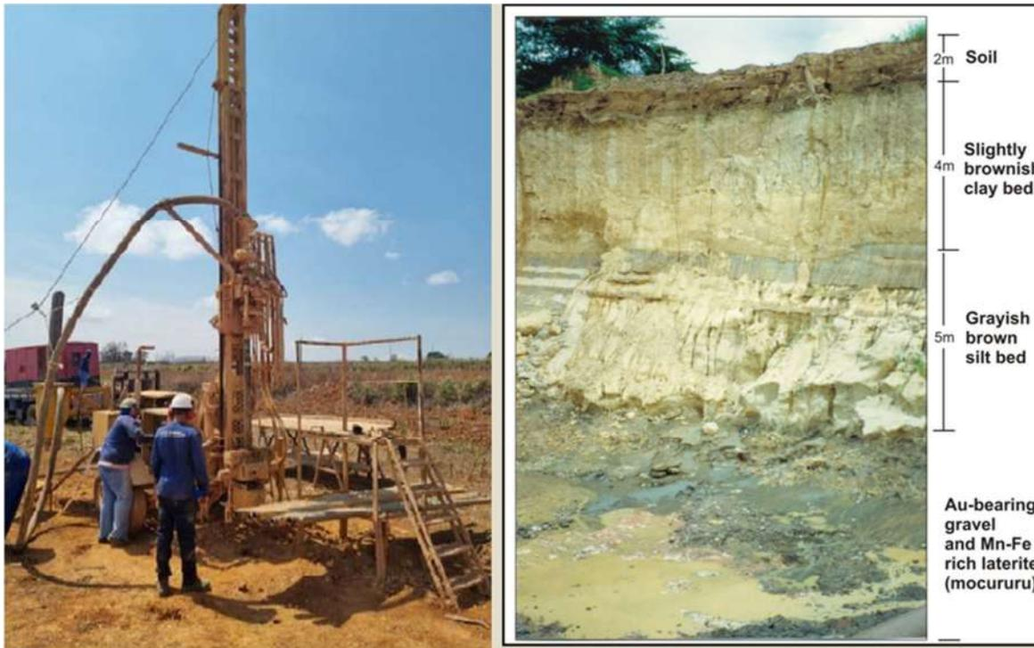
Figure 2 – Photograph of the Air Core Rig, currently being mobilized to Rondônia to initiate drilling at Canary Gold's Madeira Project. The right image shows an example of the targeted geological section of the drilling program.
