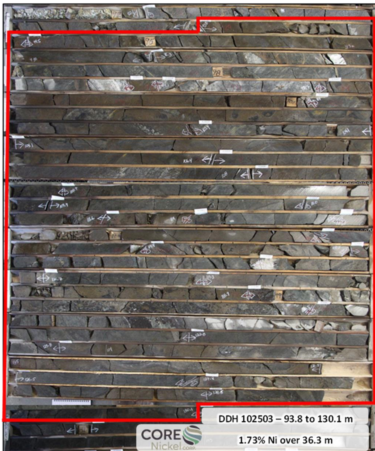
Figure 4. Nickel Intercept from Drillhole 102503 (1.73% Ni over 36.3 m)
