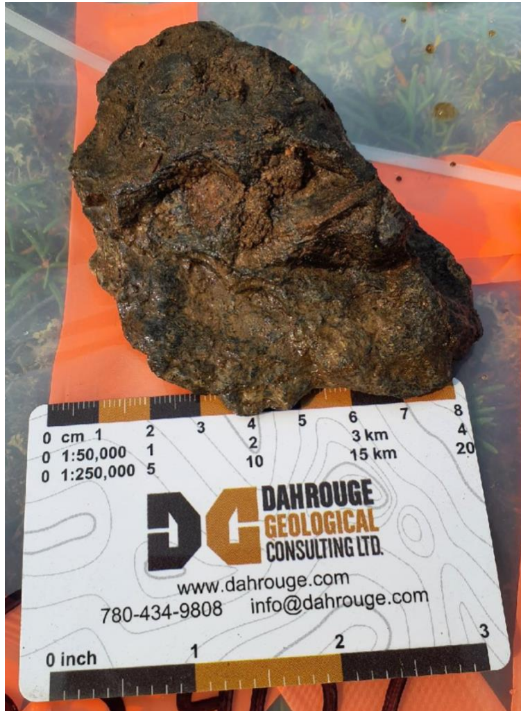
Figure 2 – Nut Lake Property Tundra - Sample 153407 - 19.69% U_3O_8 , float fragments
