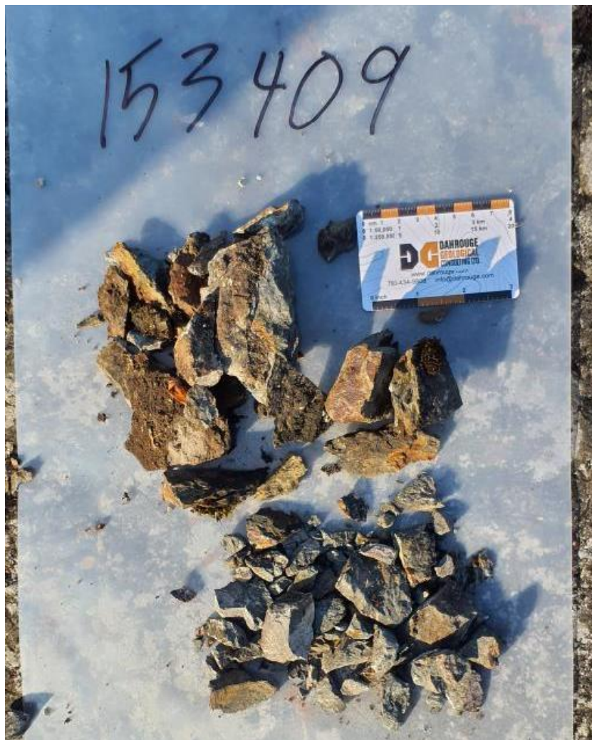
Figure 5 – Nut Lake Property Lakeshore – Sample 153409 - 0.102% U_3O_8 , 2420 ppm Ag, 1.47% Ni
