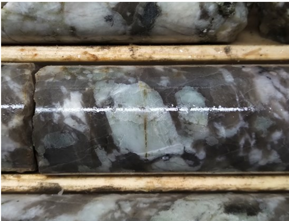
Figures 3-4: Spodumene crystal fluorescent under UV light (365nm) and light green spodumene crystal under natural light
