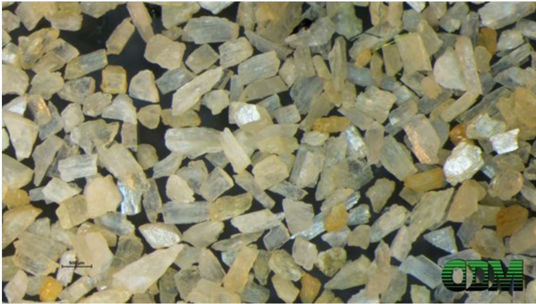
Figure 3: Grains of spodumene in till sample fraction 0.25 - 0.50mm from the Western prospect (courtesy of Overburden Drilling Management)
