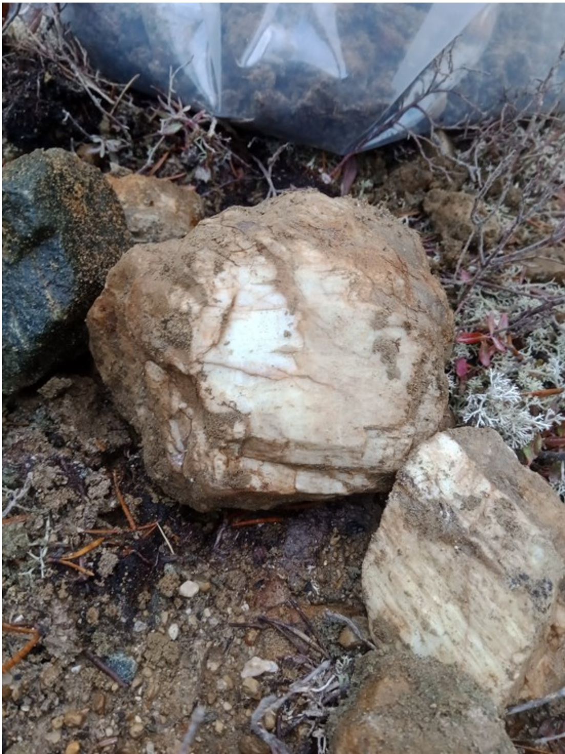
Figure 3: Fist-sized angular spodumene boulders retrieved from a till sample at the Western prospect (courtesy of IOS Services Geoscientifiques)
