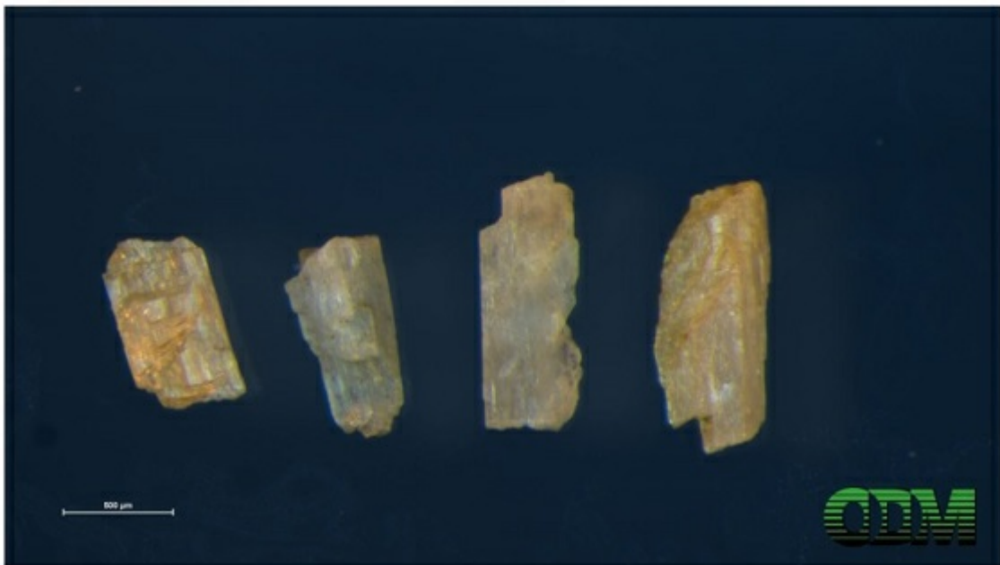
Figure 2: Grains of spodumene in till sample fraction 0.25 - 0.50mm from the Western prospect (courtesy of Overburden Drilling Management)
