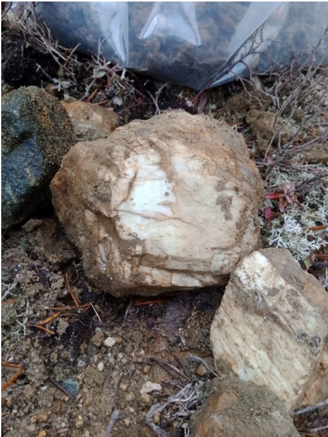
Figure 2: Fist-sized angular spodumene boulders retrieved from a till sample at the Western prospect (courtesy of IOS Services Geoscientifiques)
