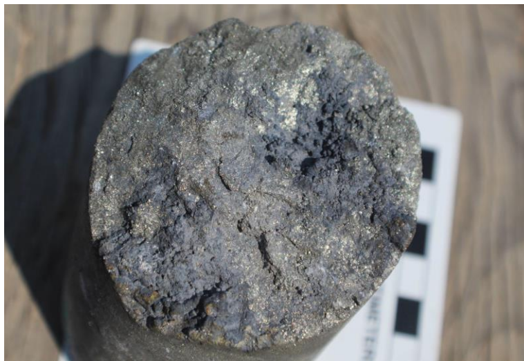
Figure 3: 2021 Drilling DDH-21-03 showing a vein with pyrite and sulfosalt minerals
