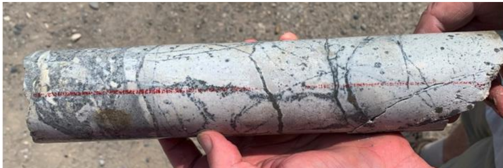
Figure 1: Drill Core from DDH-CC-21-02 showing fracture veinlets and narrow veins of sulfides
