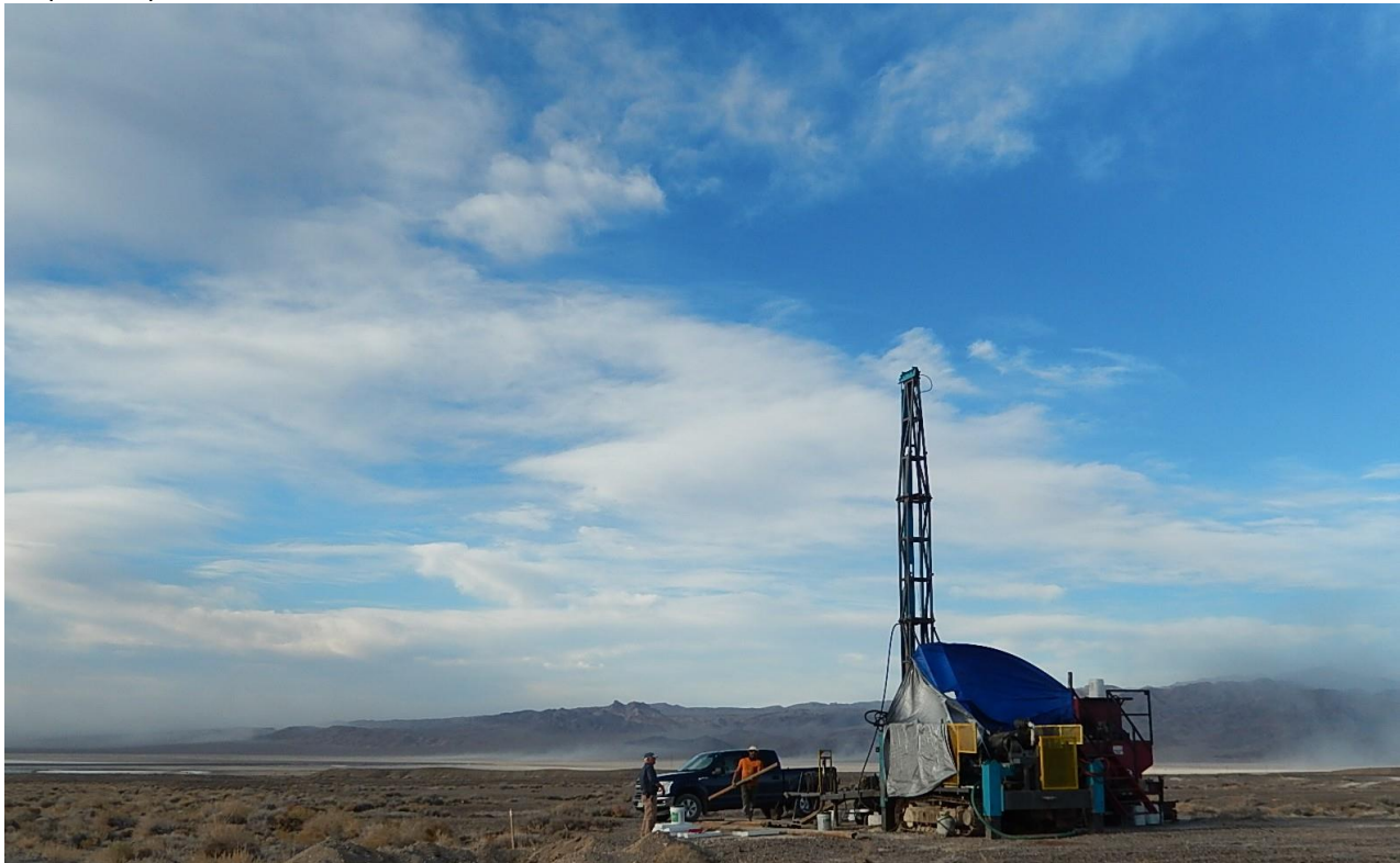
Figure 1 - LF-70 drill rig on CVZ-62 site, 2020-11-17, Brad Peek, Senior Geologist and Q.P. on site, looking northwest. CVZ-62 has 50 meters of lithium claystone and is continuing to drill in the claystones. Samples have been submitted to ALS laboratories for analysis.
