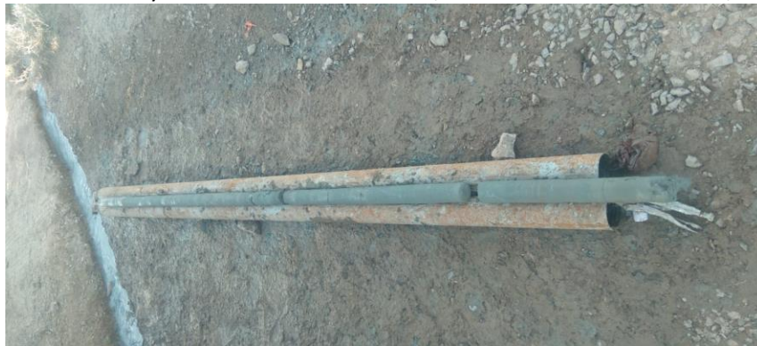
Image 1 – a portion of the over 297ft of lithium-hosted clays from CVZ-61. Greenish-blue clays typically indicating higher levels of lithium.
