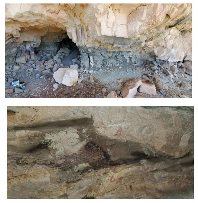
Figures 3 and 4 – The Yellow Circle underground workings have many instances where vanadium mineralization is visible, denoted by the dark grey to black coloration.
