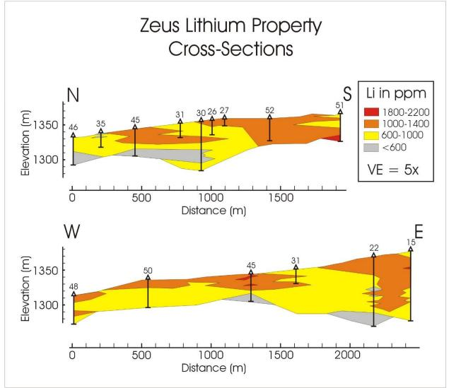
Figure 2. Zeus lithium deposit cross sections, with drill holes labeled (see figure 1 for locations). Above: North – South cross section. Below: West – East cross-section. The lithium clays are within playa lake sediments of the Esmeralda Formation.
