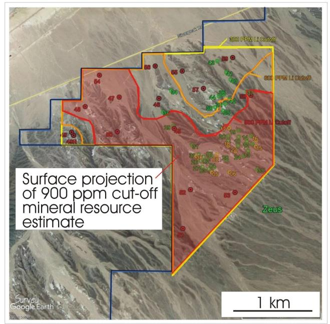
Figure 1. Google Earth image showing the area underlain by the mineral resrouce estimate (area in red, 900 ppm Li cutoff); and the boundaries for the 300 ppm Li and 600 ppm Li cutoff sensitivity analyses (orange
