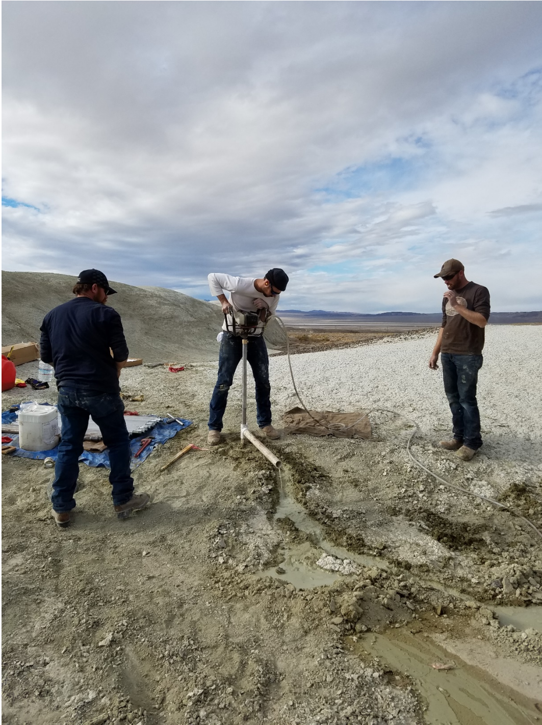
Figure 13 - Shaw Tools backpack core drill in operation on the Zeus claims.
