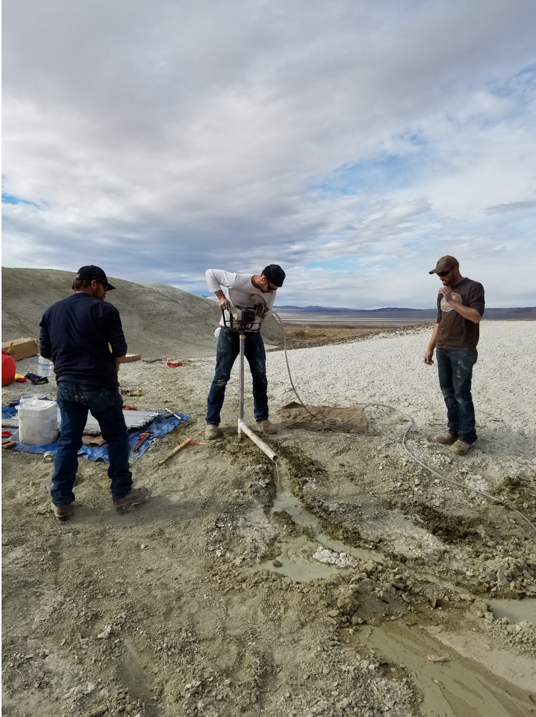
Figure 22: Shaw Tools backpack core drill in operation on the Zeus claims.
