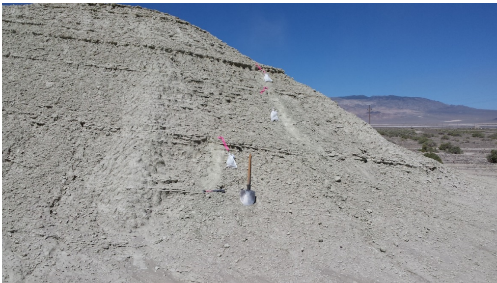
Figure 14 – Example of continuous vertical (stacked) chip samples.
