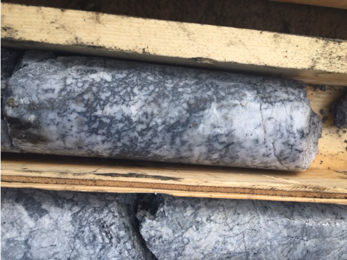
Photo description: Photos of 11.10 meter silver discovery intersection in Hole #10. Host rock is a limestone dissolution breccia/dolomitization breccia with weak to moderate silicification overprinting. Flooding this is milky quartz which hosts wispy veinlets of galena and blebby sphalerite at intersections of these or other veinlets.
