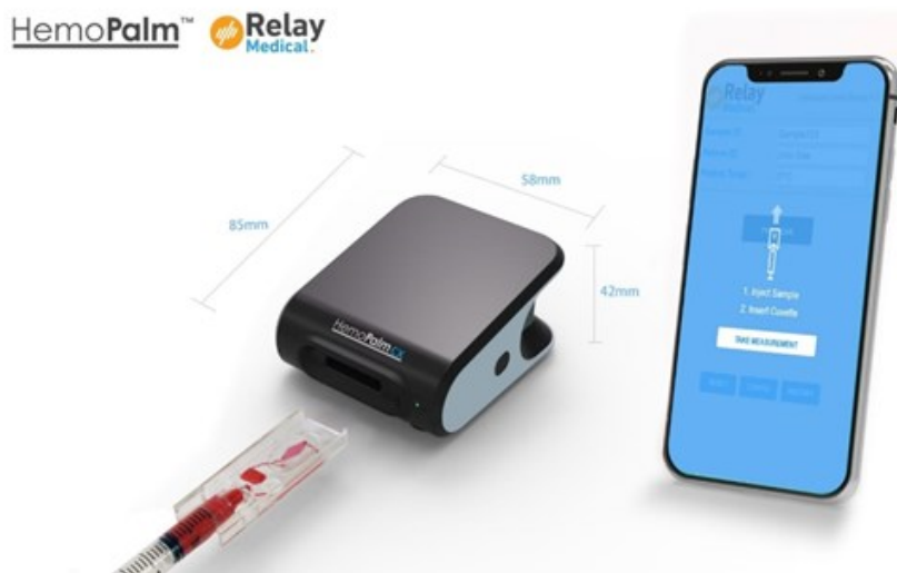
Figure 3: Concept for mini HemoPalm-CX for use with smartphone/tablet
