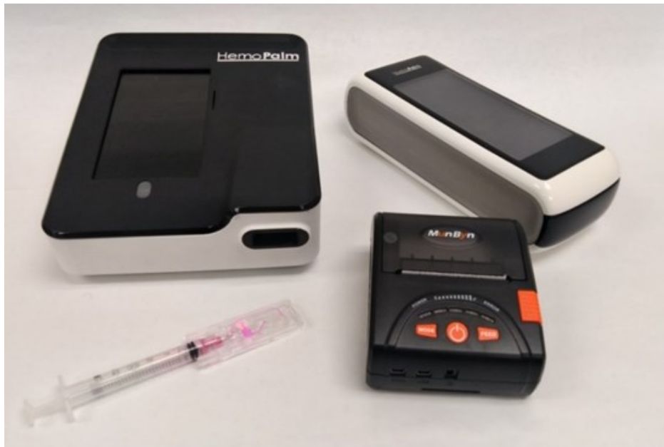
Figure 1: HemoPalm-CX Proof-of-principle prototype (left) with cartridge and portable printer (center) and mock-up of handheld instrument concept (right)
