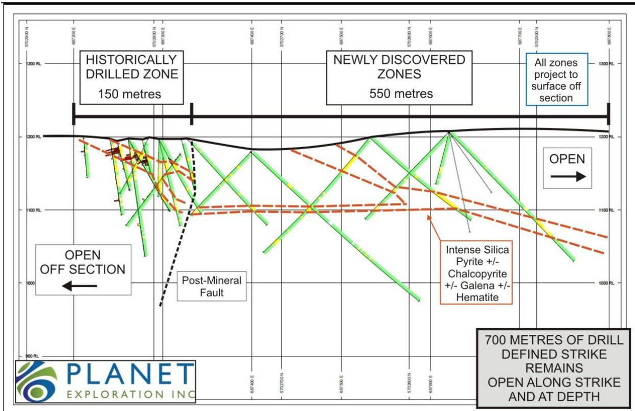
Northwest to southeast cross section through historically drilled and newly discovered zones of intense silica plus sulfide mineralization. Assay results are pending from the newly discovered zones.
