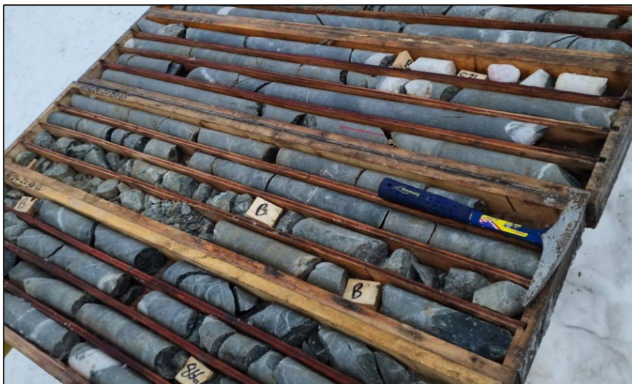
Figure 1: Altered volcanics with quartz-carbonate+/-pyrite veins to a depth of 265.2 m (870 ft) in QGQ24-20
