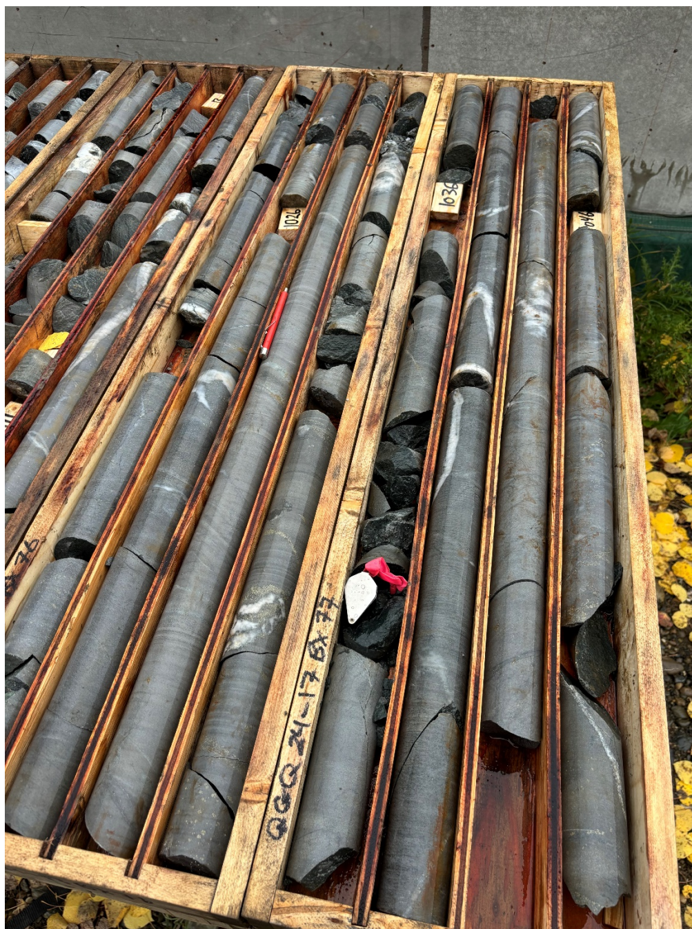
Figure 2: Photo of quartz-carbonate +/- pyrite veining and alteration observed in drill hole QGQ24-17 from a depth of 307.3 (1008.2 ft) to 319.2 m (1047.2 ft).
