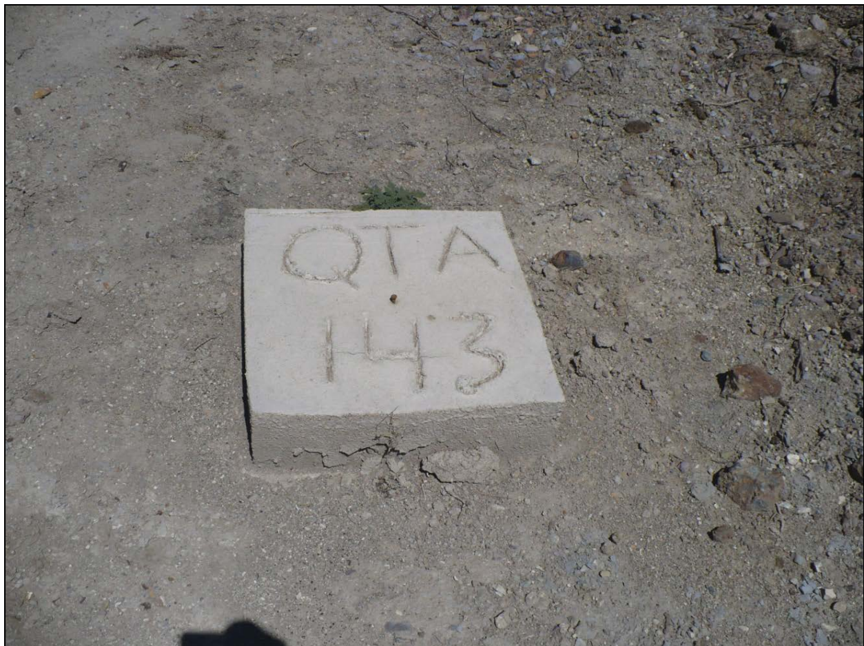
Figure 10-1: Typical Drill Hole Cap and Marker
