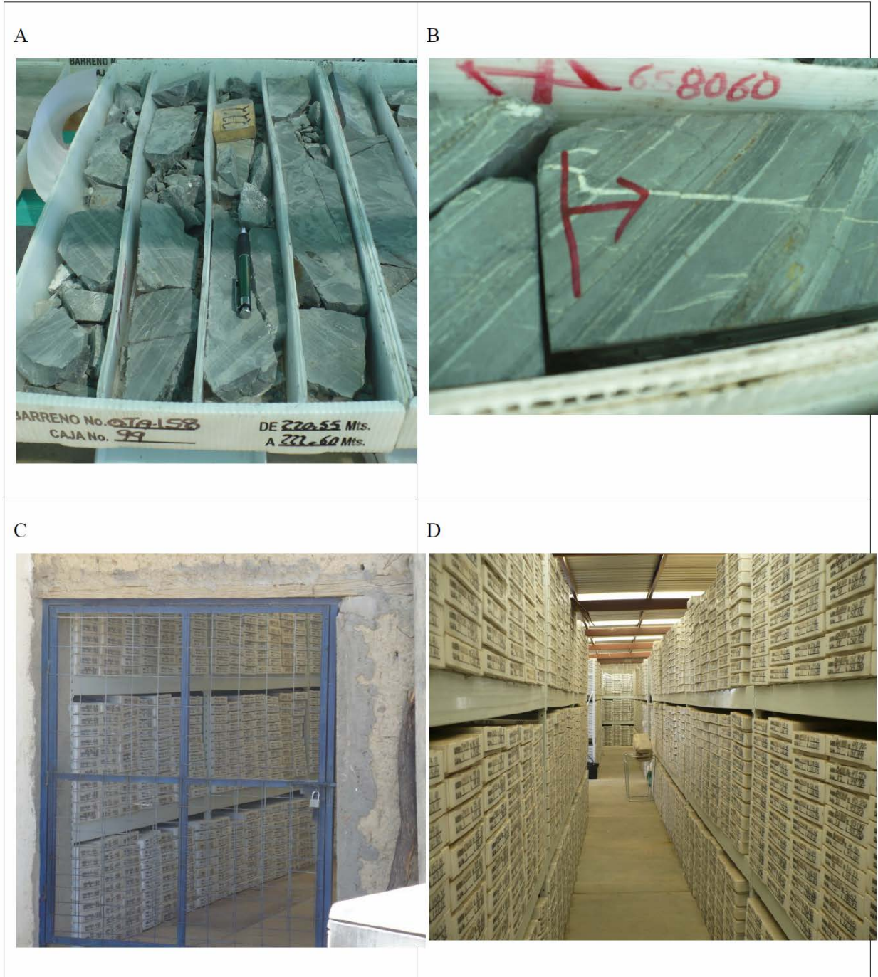
Figure 10-4: A) Core tray marked with hole ID, depth to-from of core and box number; B) typical sample ID marking in core box; C) Locked core storage 1 of 5; D) Core storage.
