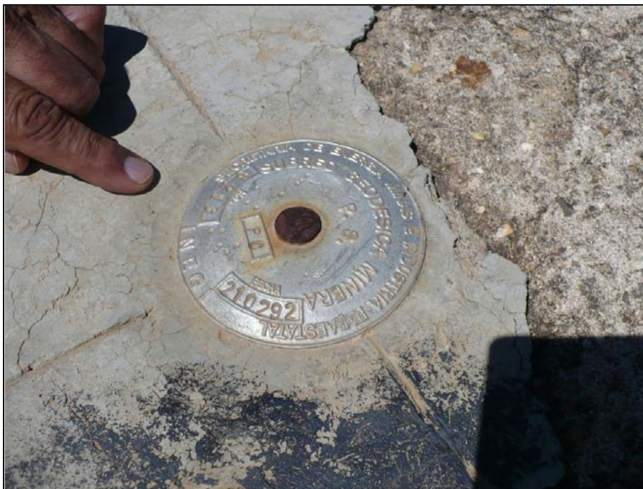
Figure 12-5: Federal survey claim marker with datum peg showing date, datum and federal identification number
