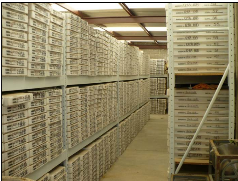
Figure 12-2: Core storage by hole and depth
