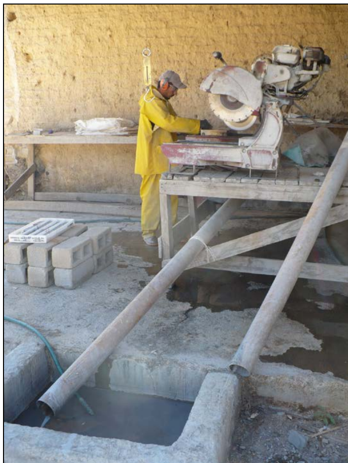
Figure 11-1 Core Cutting and sample prep area at core logging / core storage facility (Photo by Doris Fox)
