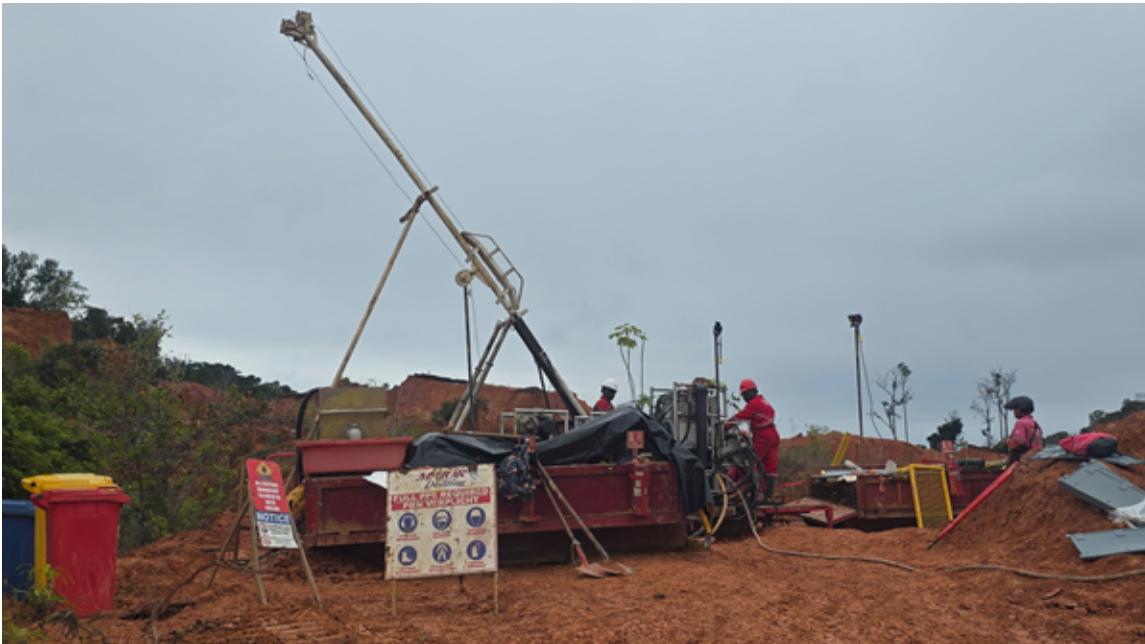
Figure 1. Drill rig and crew operating at the Stranger target on the Sela Creek Gold Project, Suriname.
