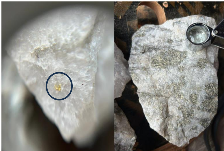
Figure 1. Grab samples at the Puma target, showing visible gold (left, field of view roughly 2 cm) and sulphides in quartz (right),
