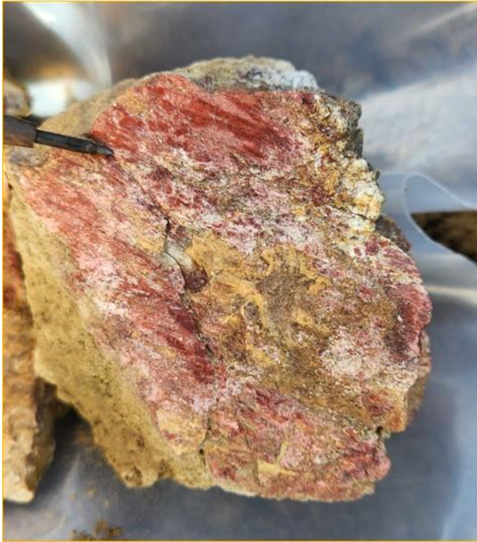
Figure 3- Sample K140214 showing intensely hematite-altered basalt with quartz-calcite stringers. Contains 111.5 ppm Cu.
