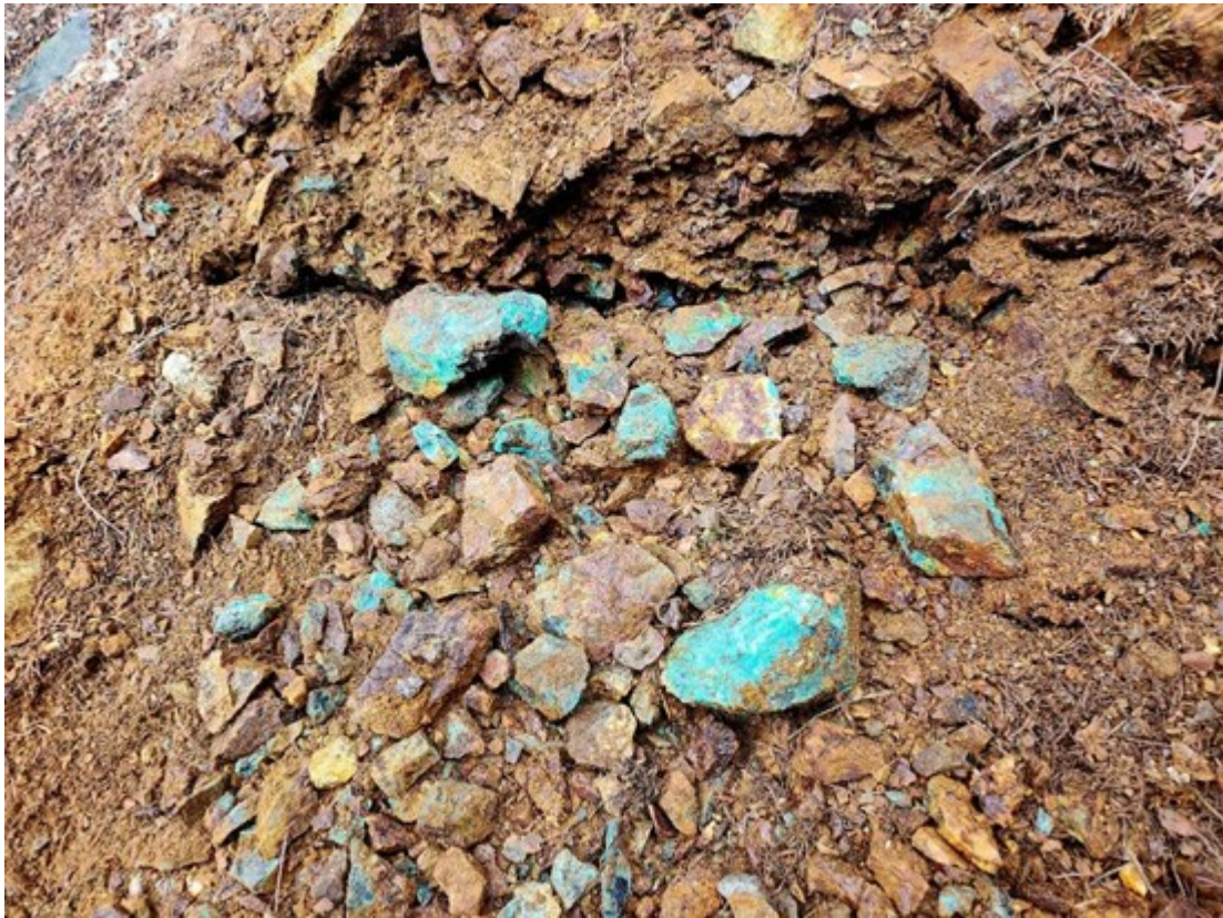
Photograph 2 - Close up of waste rock at Santana, copper oxidization evident.
