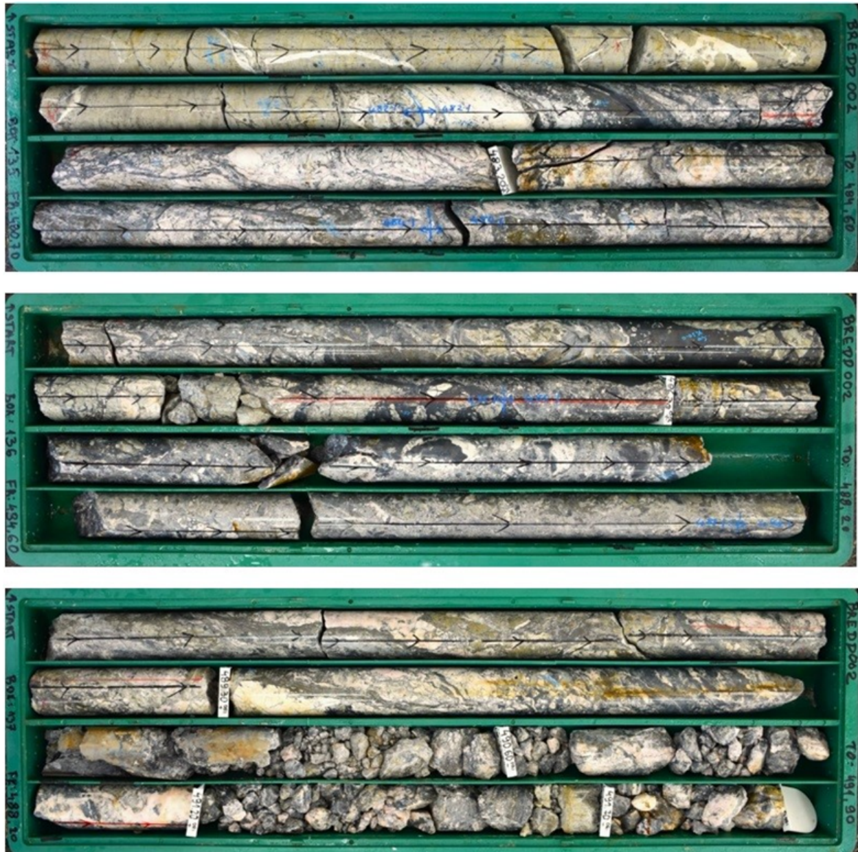
Figure 1. Photographs of three HQ3 diameter core boxes between 480.7 – 491.9 m in BREDD002. Photographs show the consistently well mineralized epithermal system which grades inwards from ginguero banded chalcedonic quartz-rhodochrosite-calcite-sulphide on the vein margins to a base metal rich central domain consisting of stibnite-sphalerite and minor galena breccia cement. Breccia is host to mineralized clasts of banded veins indicating multiple episodes of mineralization and boiling ( click here to view image ).
