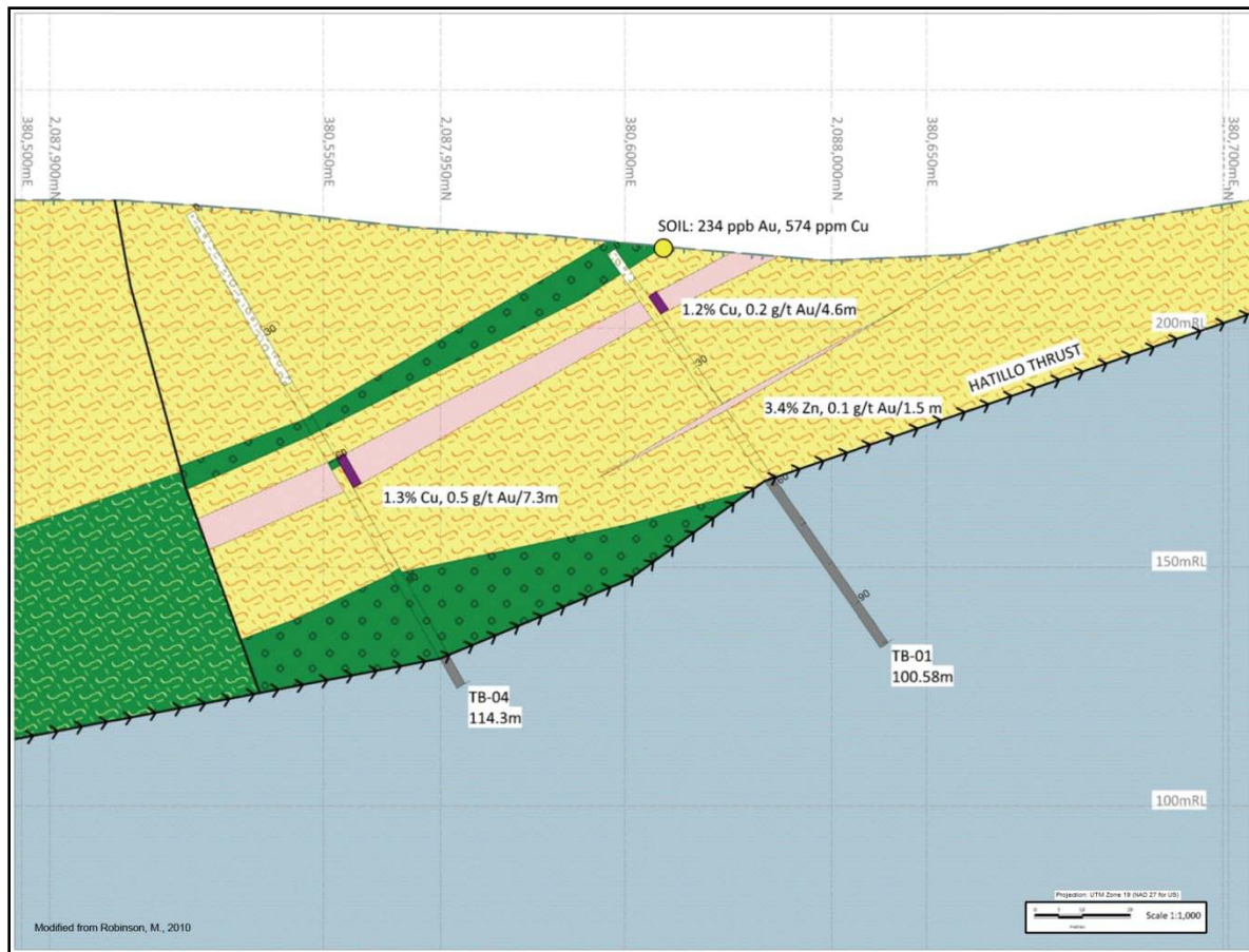
Figure 8: Schematic cross-section in the Tres Bocas prospect, Looking NW, legend in Figure 4
