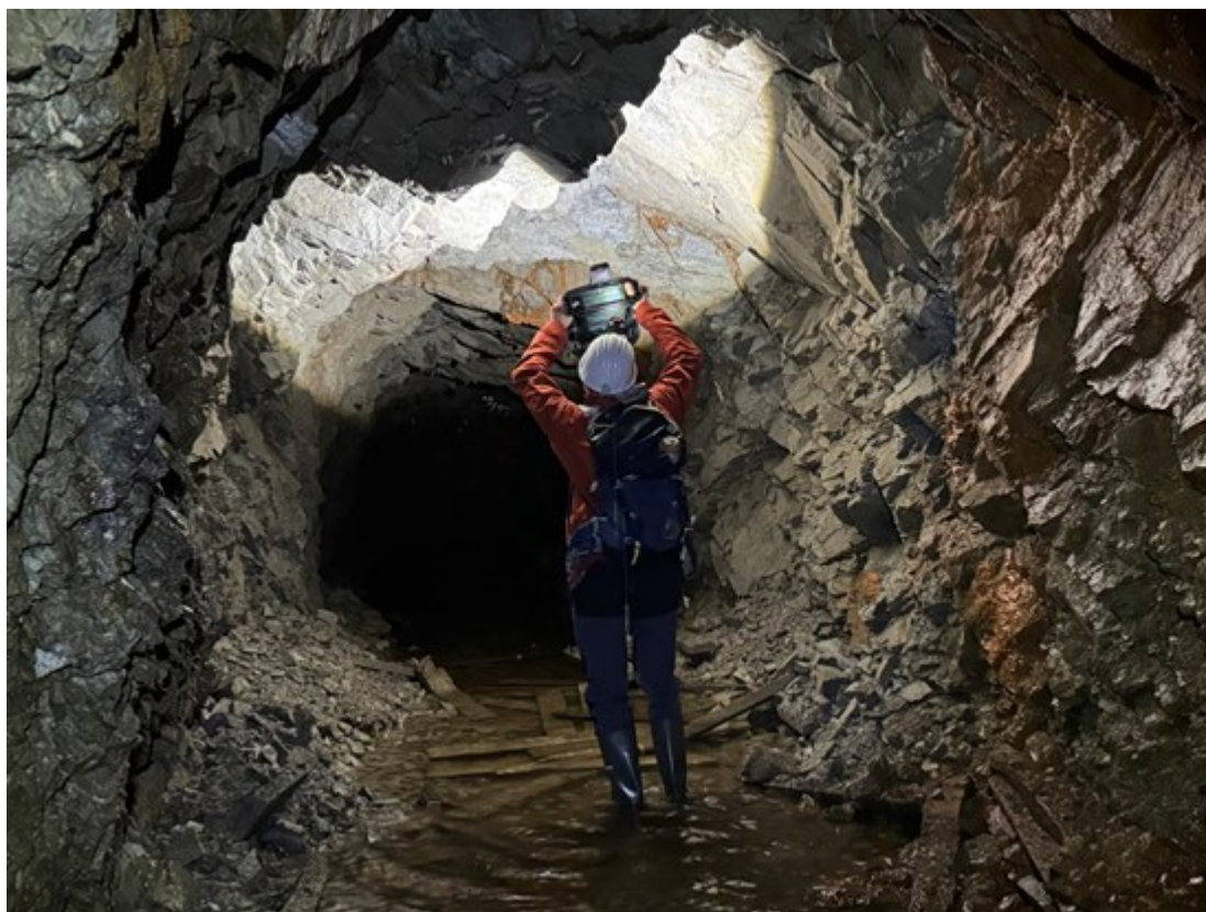
Figure 1: Military Metal's technical team conducting LIDAR survey at Trojarova
