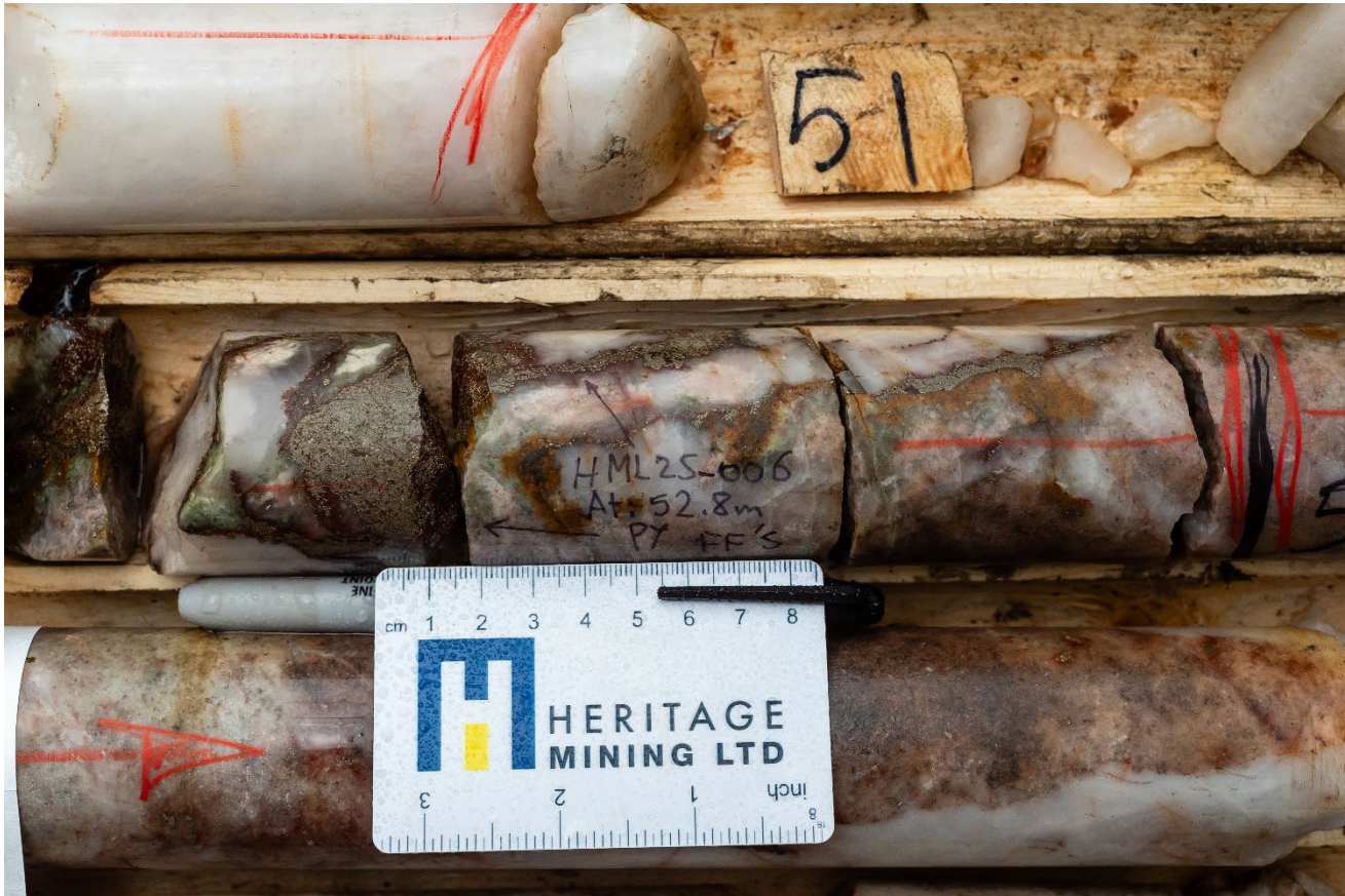
Figure 1: HML25-006 Select photograph showing variably mineralized shear zone material hosting semi massive fine grade pyrite filling laminations within massive to semi massive quartz veins associated with k-feldspar altered granite.
