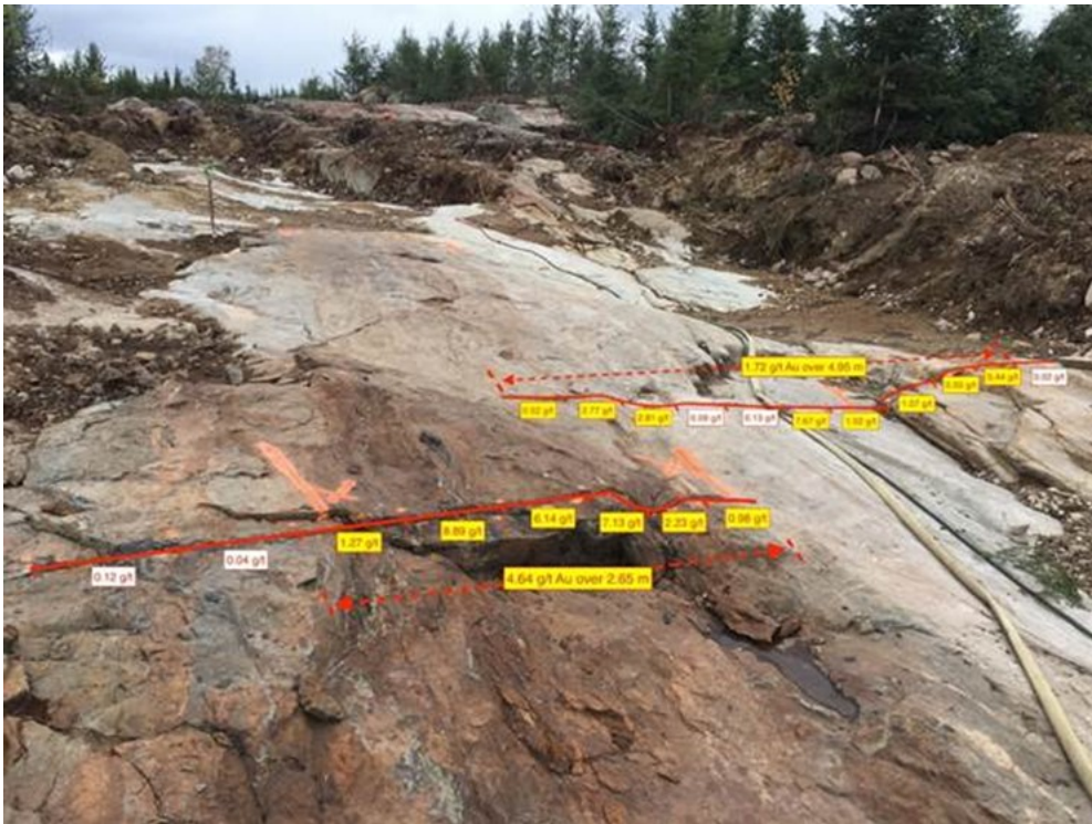
Figure 4. Field photograph of a trench that has been channel sampled at the Laird Lake property. Channel samples results are highlighted and show 4.64 g/t Au over 2.65m and 1.72 g/t Au over 4.95m.
