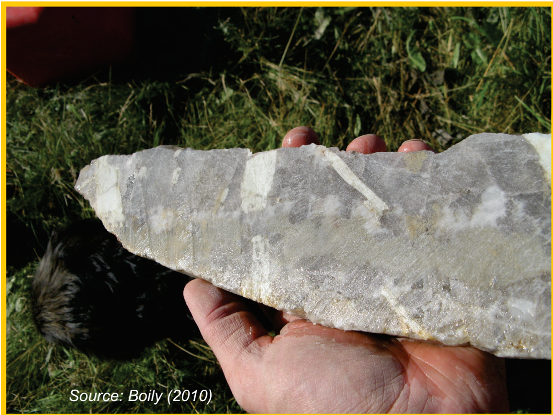
Figure 13a. White laths of spodumene with feldspar, quartz and muscovite. Bouvier showing. UTM Coord.: Easting: 714525; Northing:5370634; NAD83; Zone 17N.
