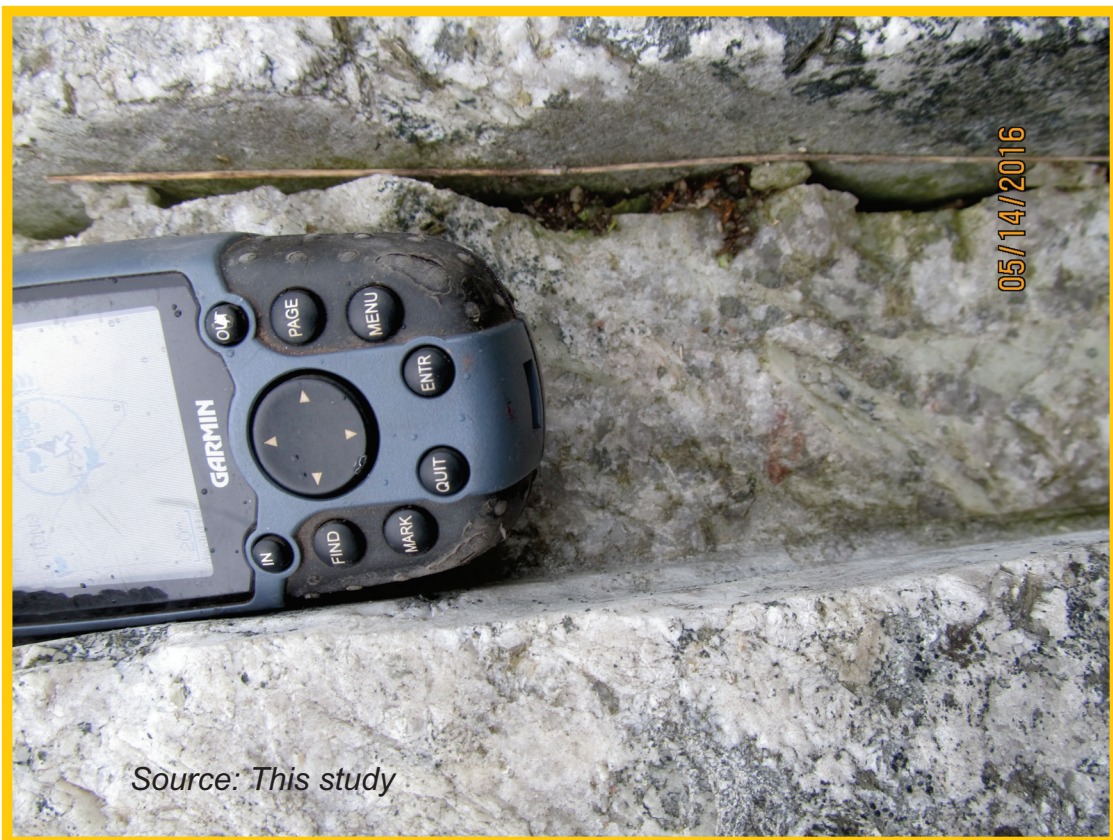
Figure 13b. Channel sample in a spodumene-bearing granitic pegmatite taken in 2009 by the geologists of Mineral Hill Industries. See the greenish laths of spodumene and pinkish garnet corresponding to sample 24752. Bouvier property. UTM Coord.: Easting: 714523; Northing: 5370634; NAD83; Zone 17N.
