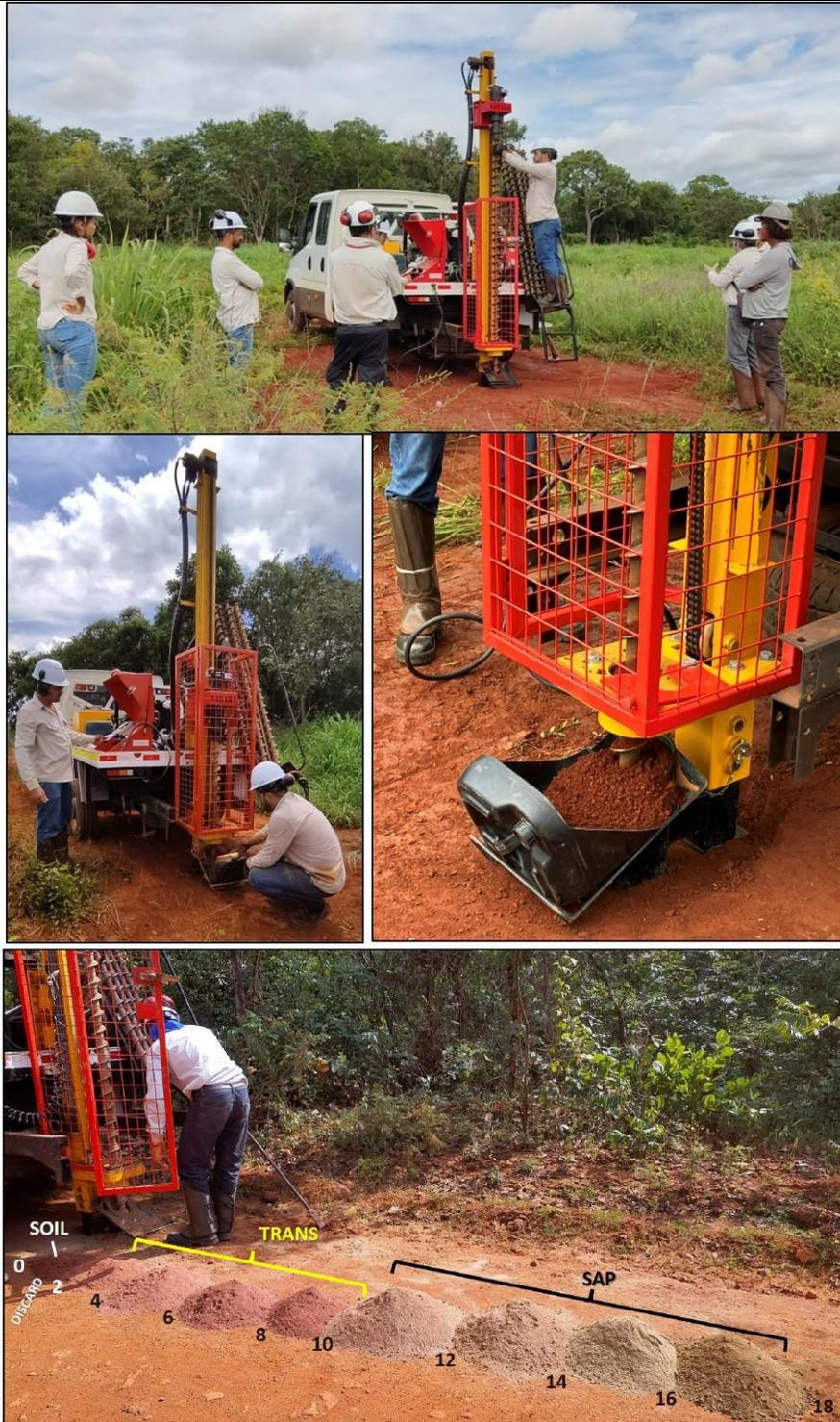
Figure 2: Images of the Truck mounted mechanical Auger Drill Rig and sampling techniques to be used at Copeçal to advance litho-geochemical modeling of the East and West Targets
