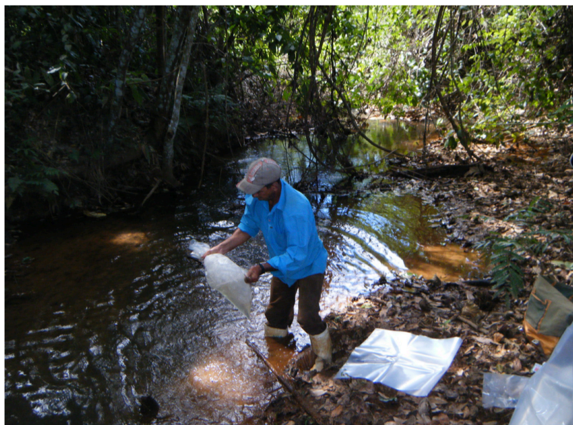
Figure 2: Stream Sediment Sampling on Copeçal Gold Project
