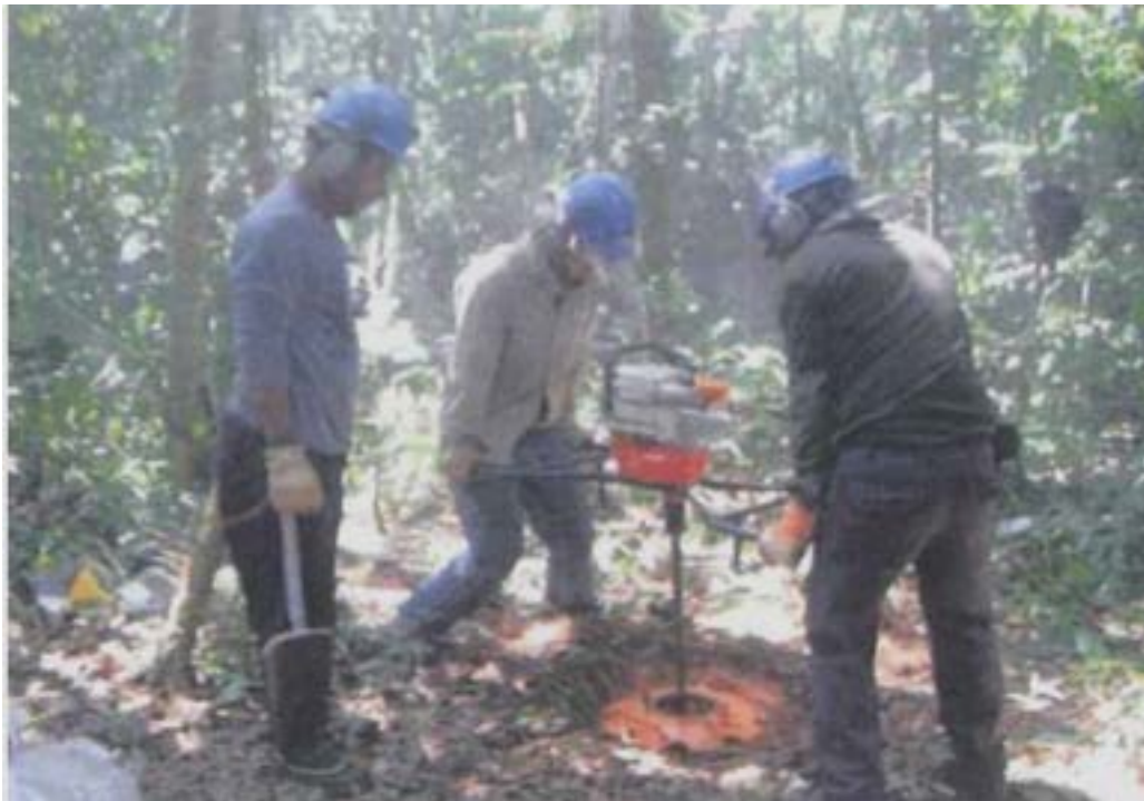
Figure 10.1 Typical drilling operation of the portable mechanized auger drill
