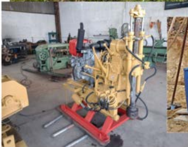
Figure 9.7 Photo of the SR-001 drill pad and the 27 hp Maquesonda 850 drill rig employed by Georras to execute drill holes SR-001 and SR-003.
