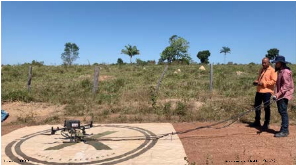
Figure 9.14 Avant DJI Matrice 300 RTK UAV/drone and attached GEM GSMP-25U magnetometer at the Copeçal Project
