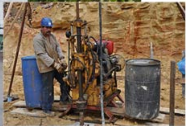
Figure 9.7 Photo of the SR-001 drill pad and the 27 hp Maquesonda 850 drill rig employed by Georras to execute drill holes SR-001 and SR-003.
