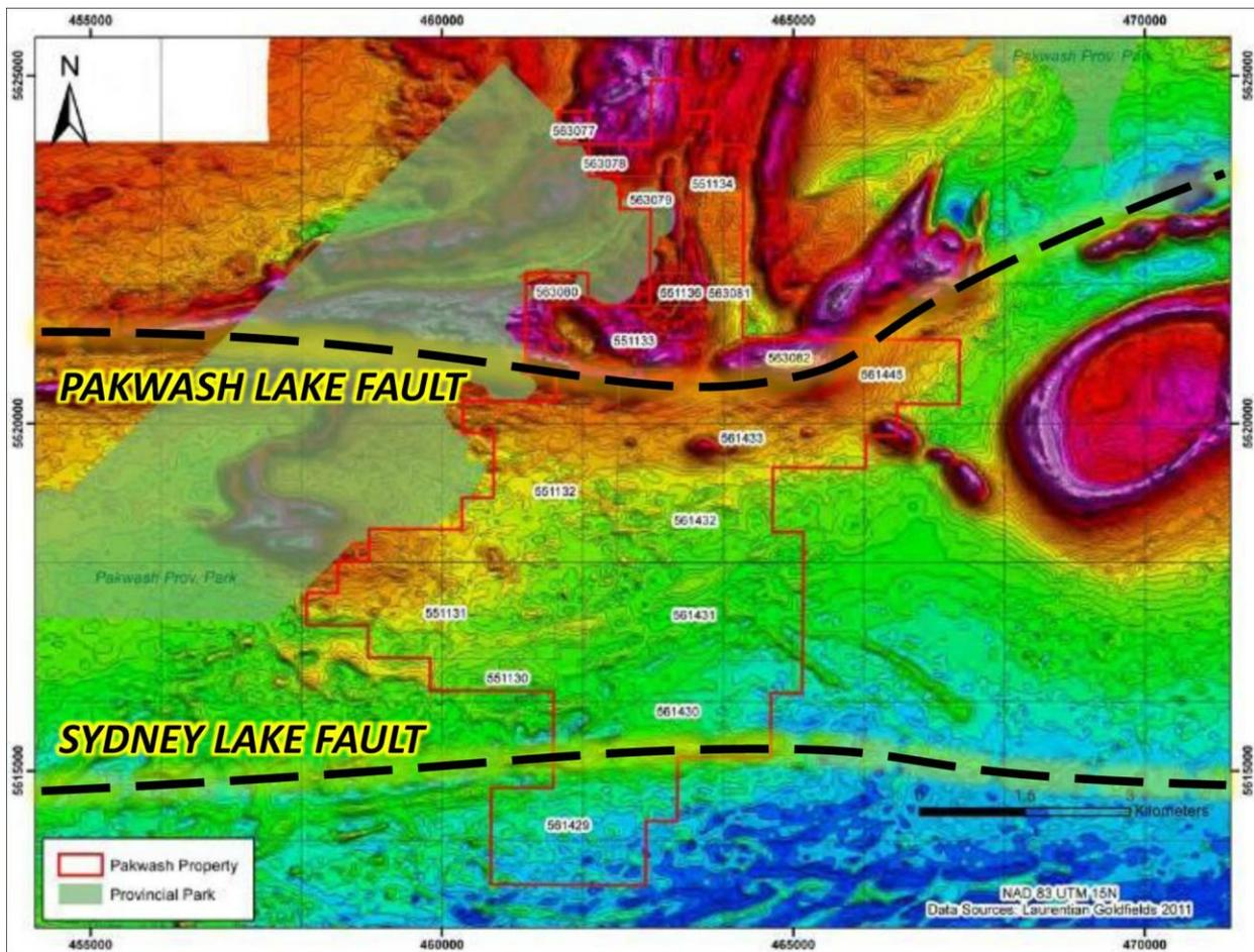
Figure 16: 2011 MAG Survey with Interpreted Tracing of the PLFZ and SLFZ Structures Crossing the Property
