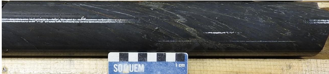
Figure 7-29 Photo 26. Folded Veinlet of Ankerite-Magnetite-Pyrite in the Aphyric Rhyolite, Drill Hole 1274-17-252 at 436 m
