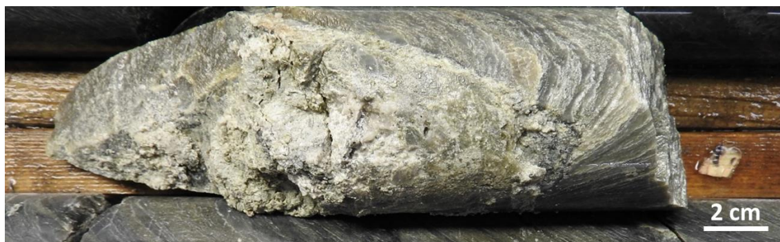
Figure 7-28 Photo 25. Decimetric-Thick Fault Cutting Through Altered Aphyric Rhyolite. The Fault Plane Has Rotated 45° Clockwise Relative to the Main Schistosity Plane When Looking Towards the End of the Hole, Drill Hole 1274-17-252 at 337 m
