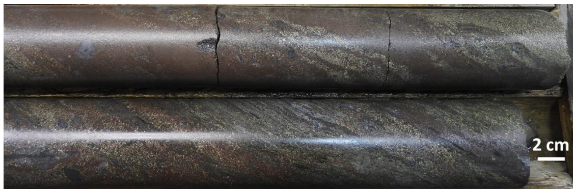
Figure 7-36 Photo 31. Lenses of Massive Sulfides (Top) to Semi-Massive (Bottom), Drill Hole 1274-17-259 at 453 m
