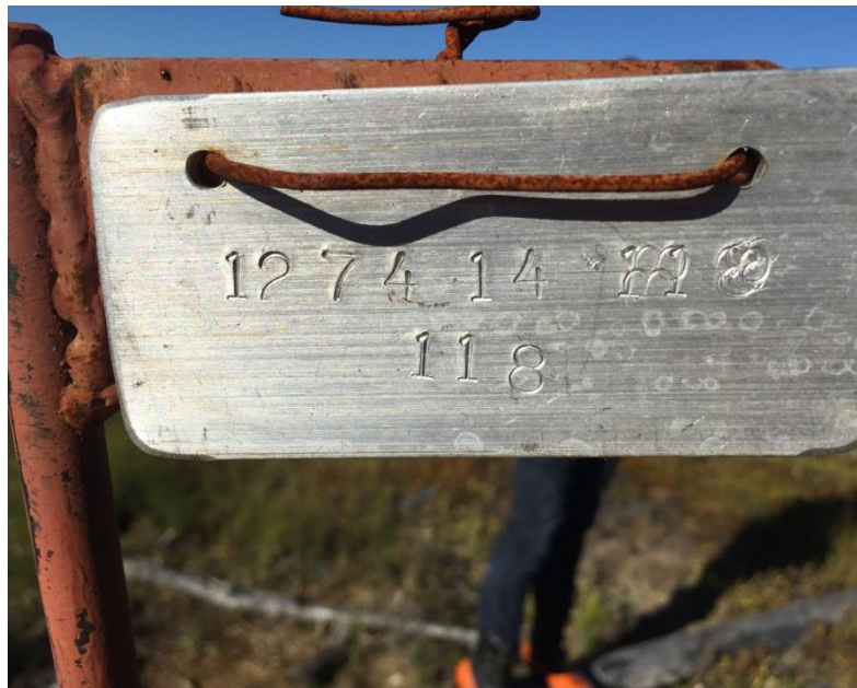
Figure 10-5 Example of Drill Marker and Identification Tag with Drilling by SOQUEM
