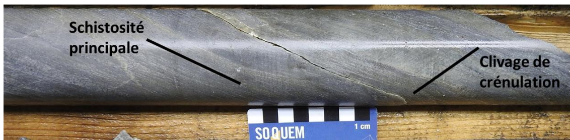
Figure 7-27 Photo 24. Main Schistosity Plane and Crenulation Cleavage in Altered Aphyric Rhyolite, Drill Hole 1274-17-259 at 420 m
