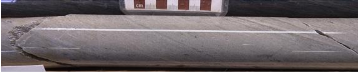
Figure 7-21 Photo 18. Felsic Aphanitic Intrusion, Weak Alteration to Chlorite-Sericite-Ankerite, Drill Hole 1274-16-224 at 216 m
