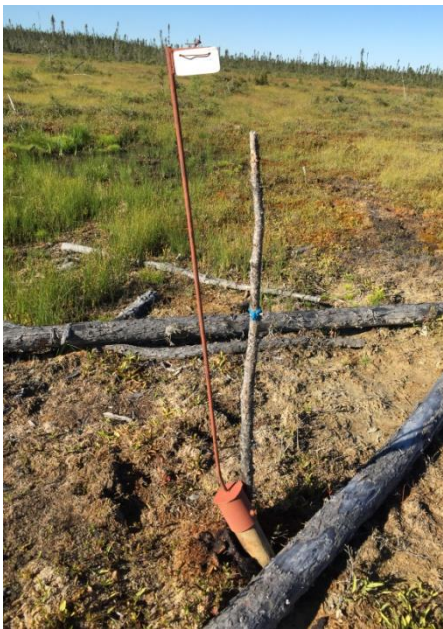
Figure 10-5 Example of Drill Marker and Identification Tag with Drilling by SOQUEM
