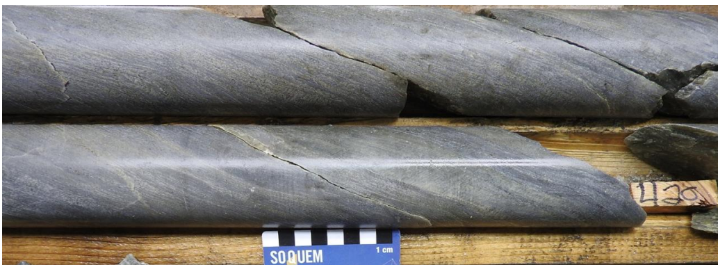
Figure 7-33 Photo 28. Intense Sericite Alteration Overlying the Brecciated Aphyric Rhyolite, Drill Hole 1274-17-259 at 420 m
