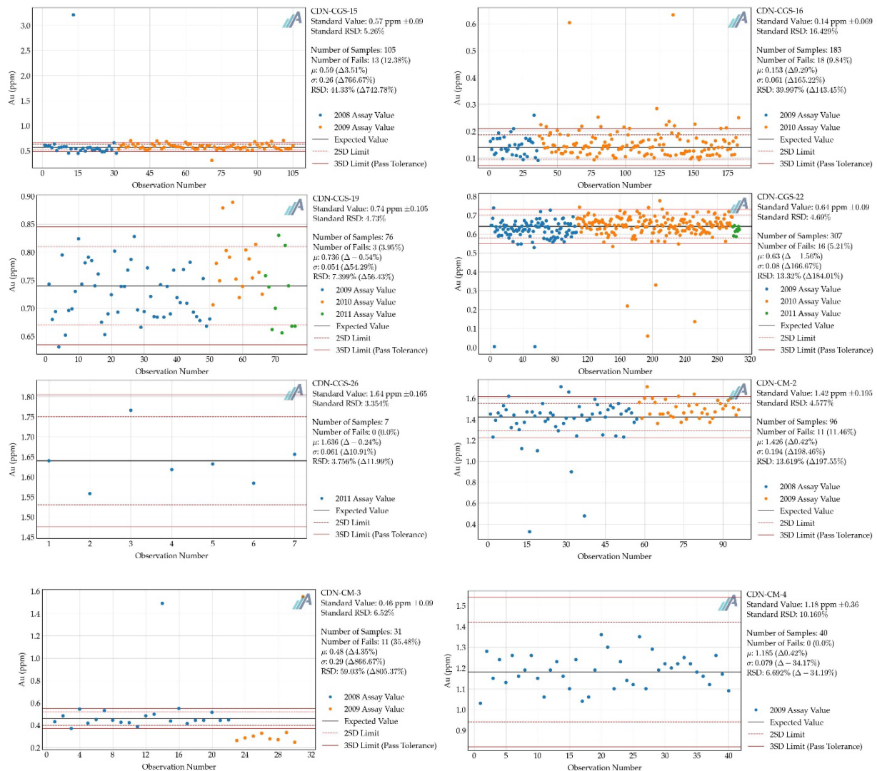
Figure 11.1 Au analysis for CRMs and blanks inserted by the operator during the 2008-2012 EVG drilling programs.
