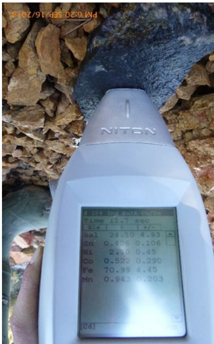
Figure 6.2. Niton XLp Portable XRF Analyzer. Analyzer is showing field reading of 2.7% Ni on magnetite vein at Commerce East.
