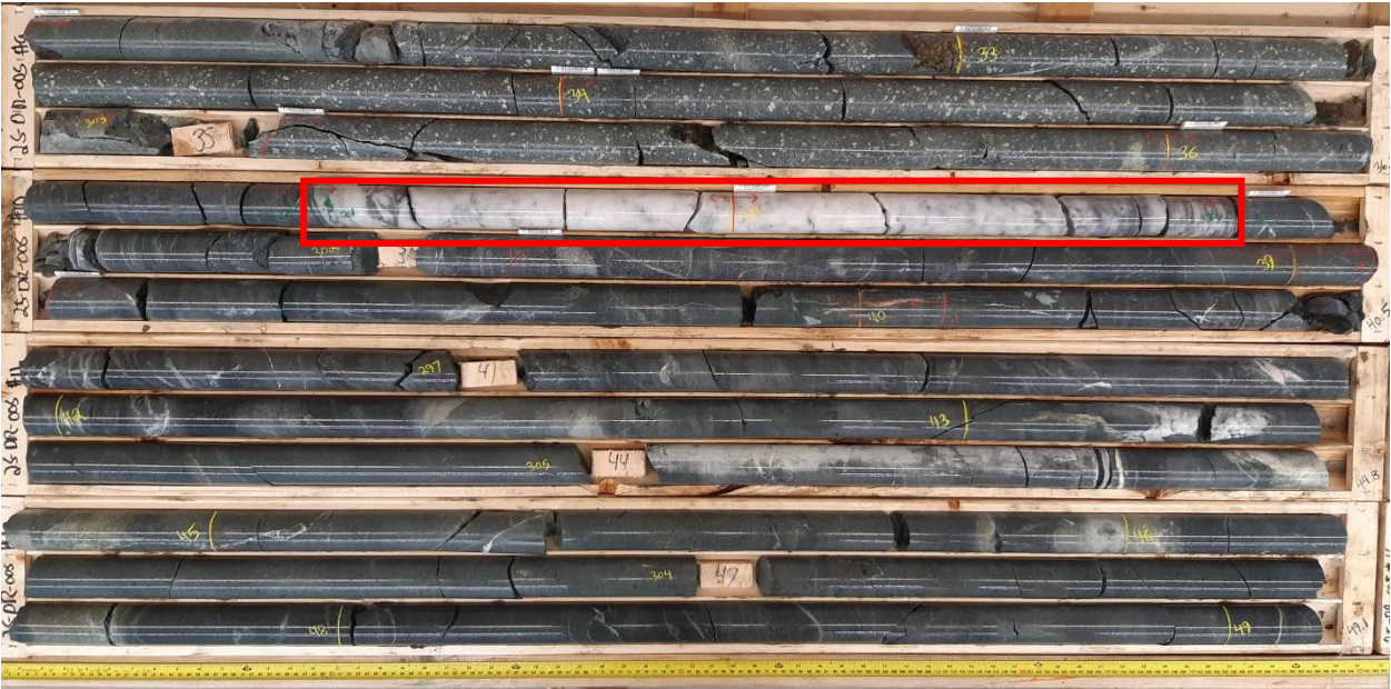
Figure 2: Hole 25-DR-005 32.0m to 49.1m, featuring a 1.1m long pyrite mineralized quartz vein from 36.5m to 37.6m downhole, outlined in red.
